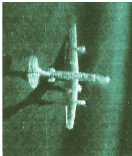
Sidescan sonar image of sunken plane in 150 feet of water
