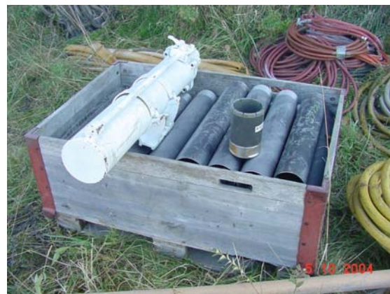
Figure 14. Two foot long casing and diamond drill bit
