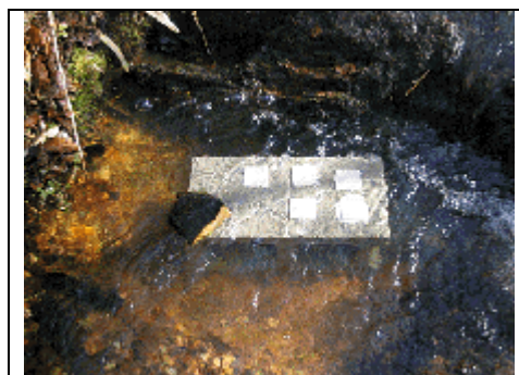
Figure 7. Unglazed ceramic streak plates deployed on a concrete block in a stream draining a gold prospect, Piedmont, North Carolina. A time-integrated field experiment to collect iron-manganese oxyhydroxide coatings with arsenic at this location. Broken natural rock (placed left corner of block) shows heavy natural iron-manganese coating on quartz rock. Six streak plates were affixed to each block plates could be removed over time and their coatings geochemically analyzed to monitor rate of iron-manganese coating development. The blocks were set so that oxygenated water ran over the top of the blocks. Eh conditions are important in precipitation of such
