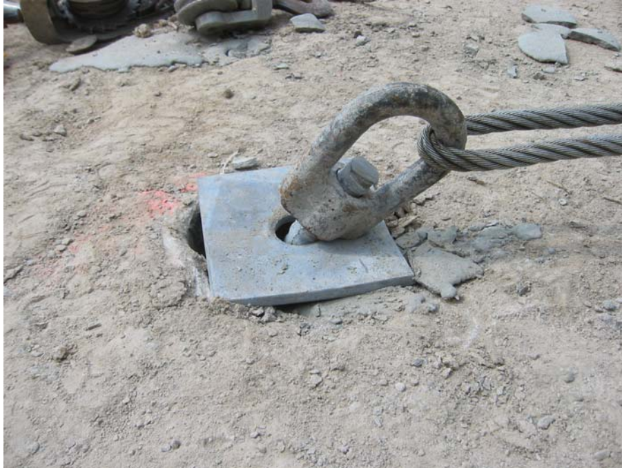
Figure 11. Test 2, vertical bar, restrained by using rock bolt faceplate. Load maintained to 11 tonnes without failure.
