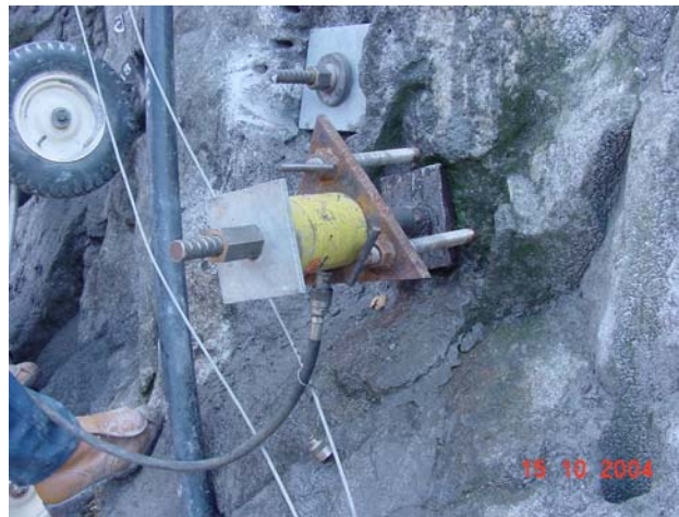
Figure 12. Lift-off test for pre-stressed rock bolts
