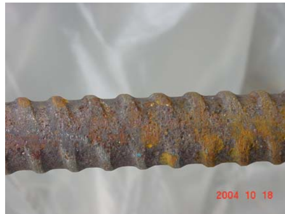
Figure 19. Pitting and cratering along rock bolt
