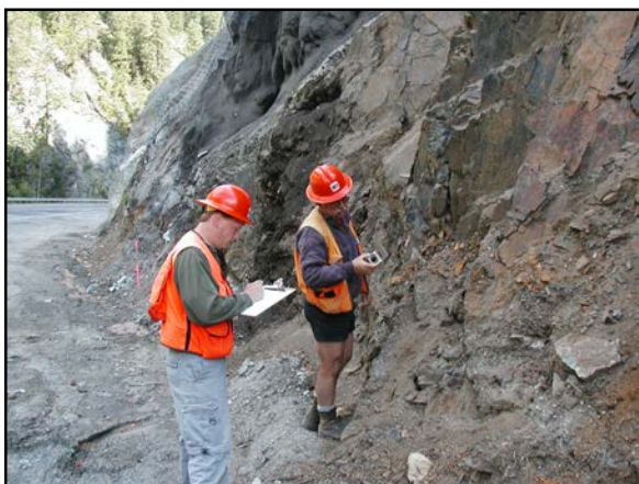
Figure 2b: Kleinfelder team mapping fractures on a rock face on SR 97 near Ruby Creek.
