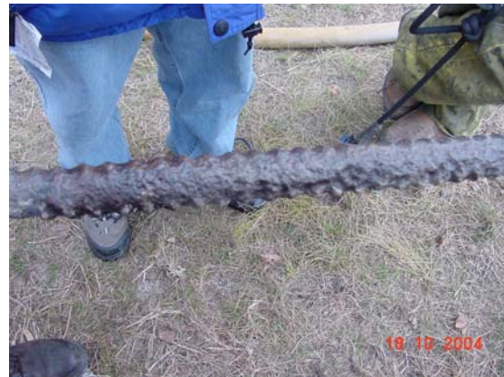
Figure 21. Corroded rock bolt
