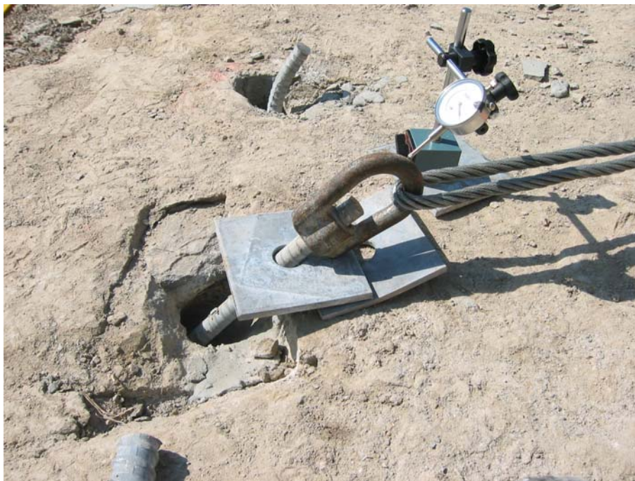
Figure 12. Test 3, inclined bar, also restrained. Load increased to 12 tonnes without failure, or notable deformation of bar.
