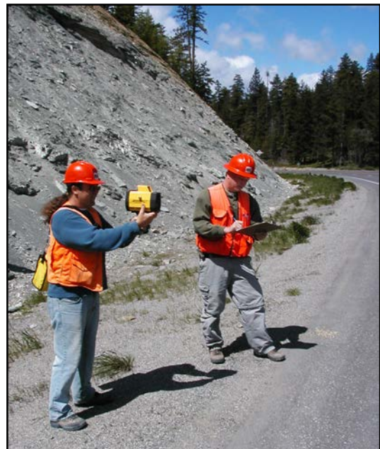
Figure 2a: Kleinfelder team employing a laser range finder to define the size of the unstable slope problem on SR 97 near Blewett Pass, Washington.
