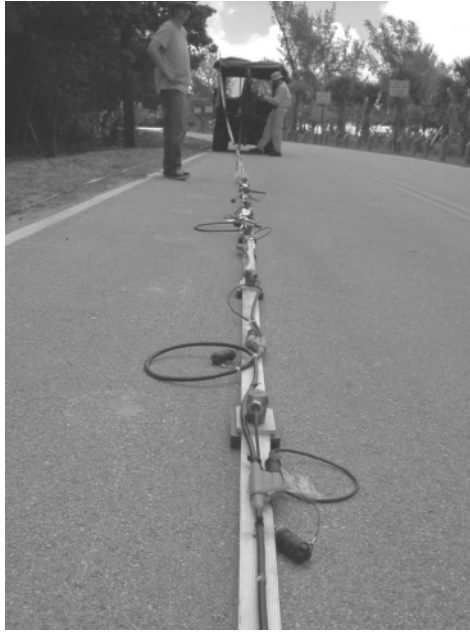
Figure 6. Landstreamer setup for a 24-geophone array pulled with an ATV along a road
