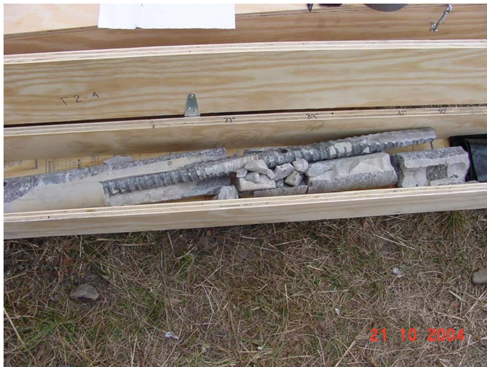
Figure 22. Recovered 1.25 inch diameter, steel tendon and cement grout
