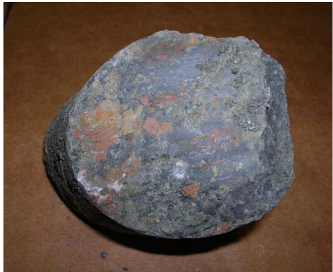
Figure 5. Slickensides found in the Lawrence Shale Formation on alignment near proposed grade on Pleasant Grove Hill.
