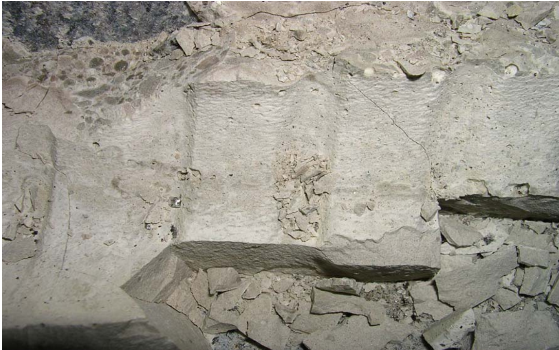
Figure 6. Pores Distributed Throughout Portland Cement Grout Sample.
