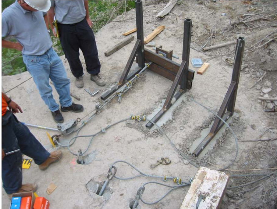
Figure 8. Four anchors installed six-days previously, reaction frame designed to be very stiff. Come-along used to take slack out of cables.
