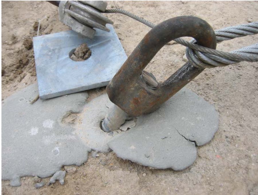
Figure 10. First pull test. Vertically installed bar had bent to 45° under 4 Tonnes load.
