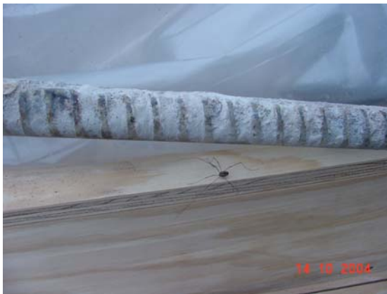
Figure 18. Rock bolt with resin grout
