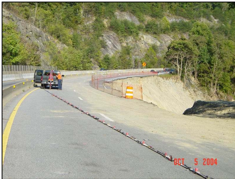
Figure 6 – MASW data acquisition along main slide on I-40 using 24-channel land streamer and AWD energy source. Photo looking east.
