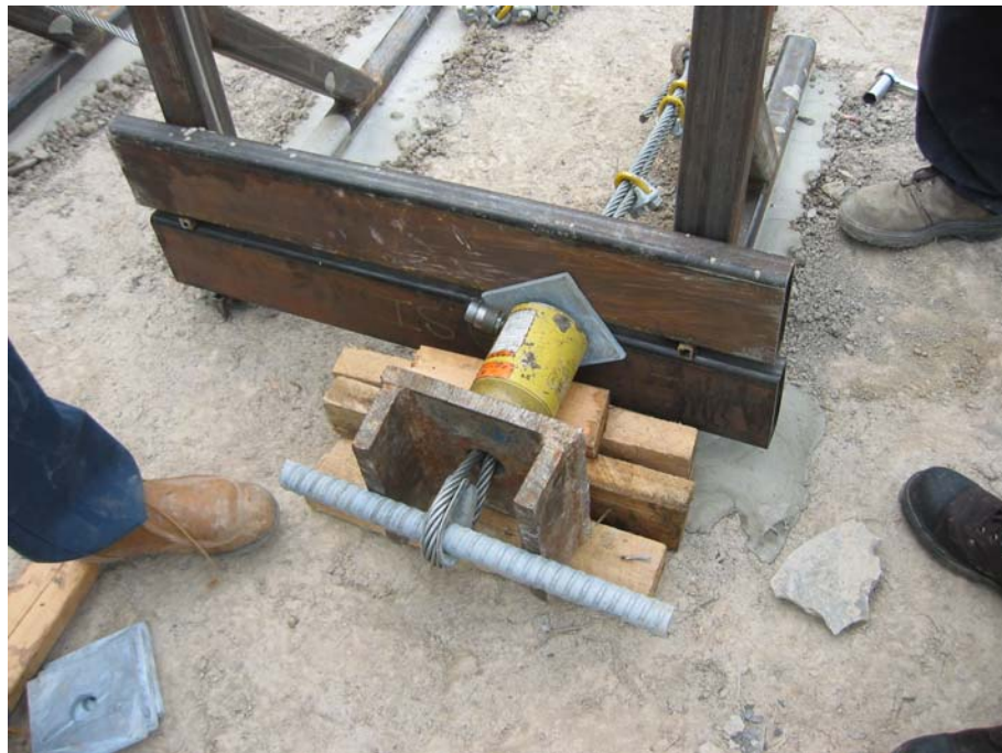
Figure 9. Loading arrangement to put cable into tension and transfer load to anchor bolt.
