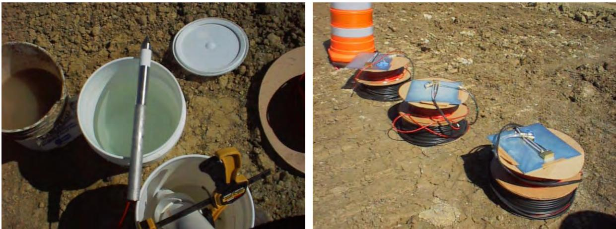
**Figure 13 – VW Piezos (left) and S-Cells (right) During Instrumentation Installation**
