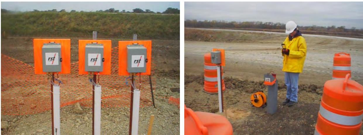
**Figure 14 – Instrument Terminal Station (left) and Monitoring of Instruments (right)**
