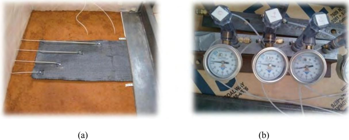
**Figure 6 - (a) Wireline extensometers attached to the geotextile and tensiometer probes near the soil-geotextile interface, (b) tensiometer readout dials**
