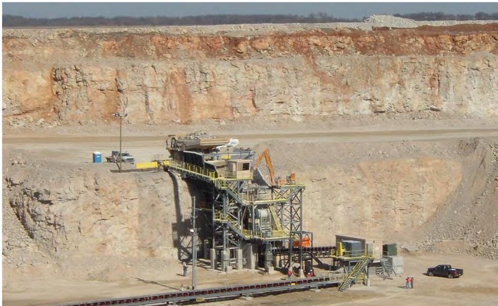
Fig. 10. Martin Marietta Materials limestone (West Spring Creek Formation) quarry near Troy, Oklahoma. Primary crusher near center of photograph.
