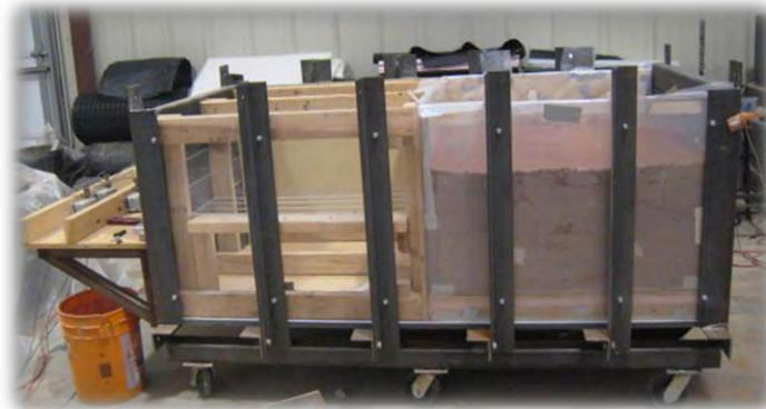
**Figure 5 – Pullout test box at the end of sample preparation.**
