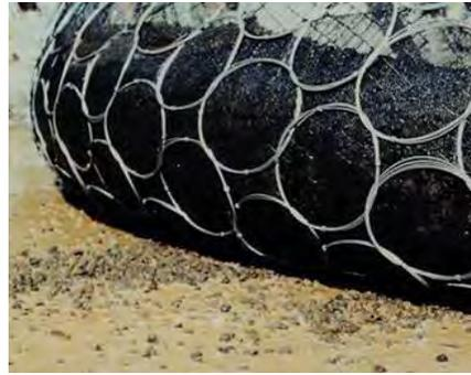
Figure 1 & 2. Debris in Ring Nets during Test Simulation in Oregon.
