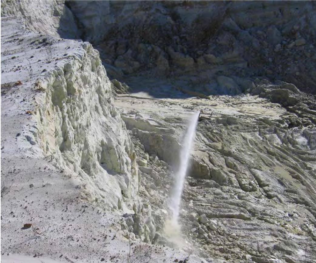
Fig. 8. Hydraulic mining of high-purity silica sand of the Oil Creek Formation in U.S. Silica Company's Mill Creek quarry.
