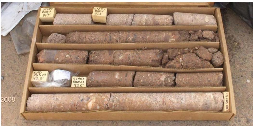
**Figure 5 – Weak Rock (Conglomerate) Typical of Stratum C Soils**
