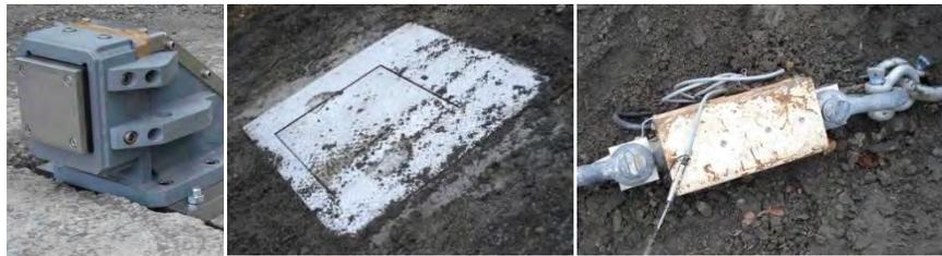
Figures 6, 7, & 8. Impact pressure sensor, force plate and force cell
