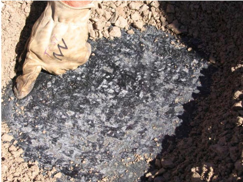
**Figure 8 – Exposing the membrane to check for punctures**
