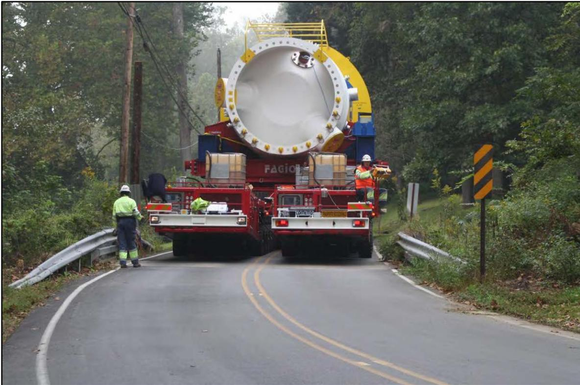
A subsurface investigation was performed with geotechnical laboratory testing to support slope stability analyses along this two-mile stretch of road. Baker looked at the load applied as a strip load much like a foundation load as well as individual and combination wheel loads for a shallow failure that could progress into a global failure. Baker found satisfactory factors of safety for all conditions investigated.
