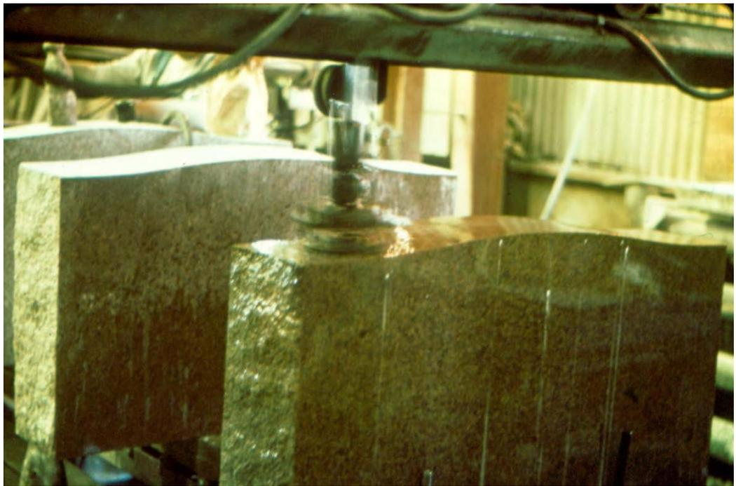
Fig. 12. (A) Granite dimension stone quarry near Troy, Oklahoma, and (B) polishing granite at Willis Granite Products near Granite, Oklahoma.
