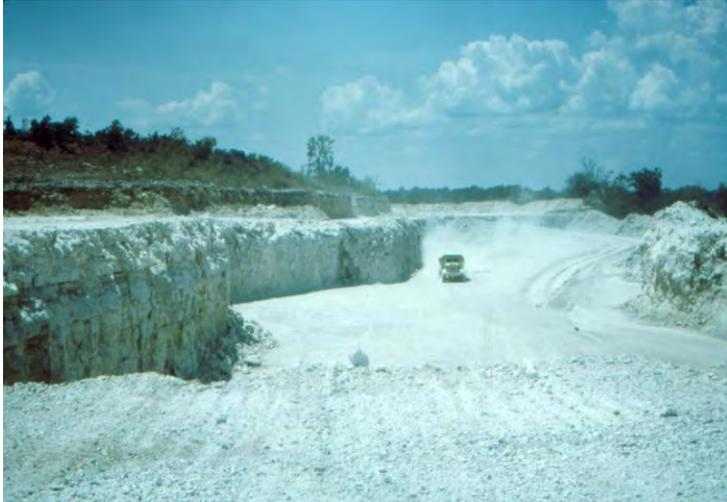
Fig. 11. The Goodland Limestone, 65 ft thick, is mined near Idabel, Oklahoma.
