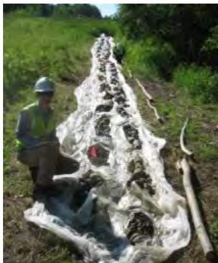
Figure 11 - Logging sonic drill continuous core samples of the overburden (June 2013).
