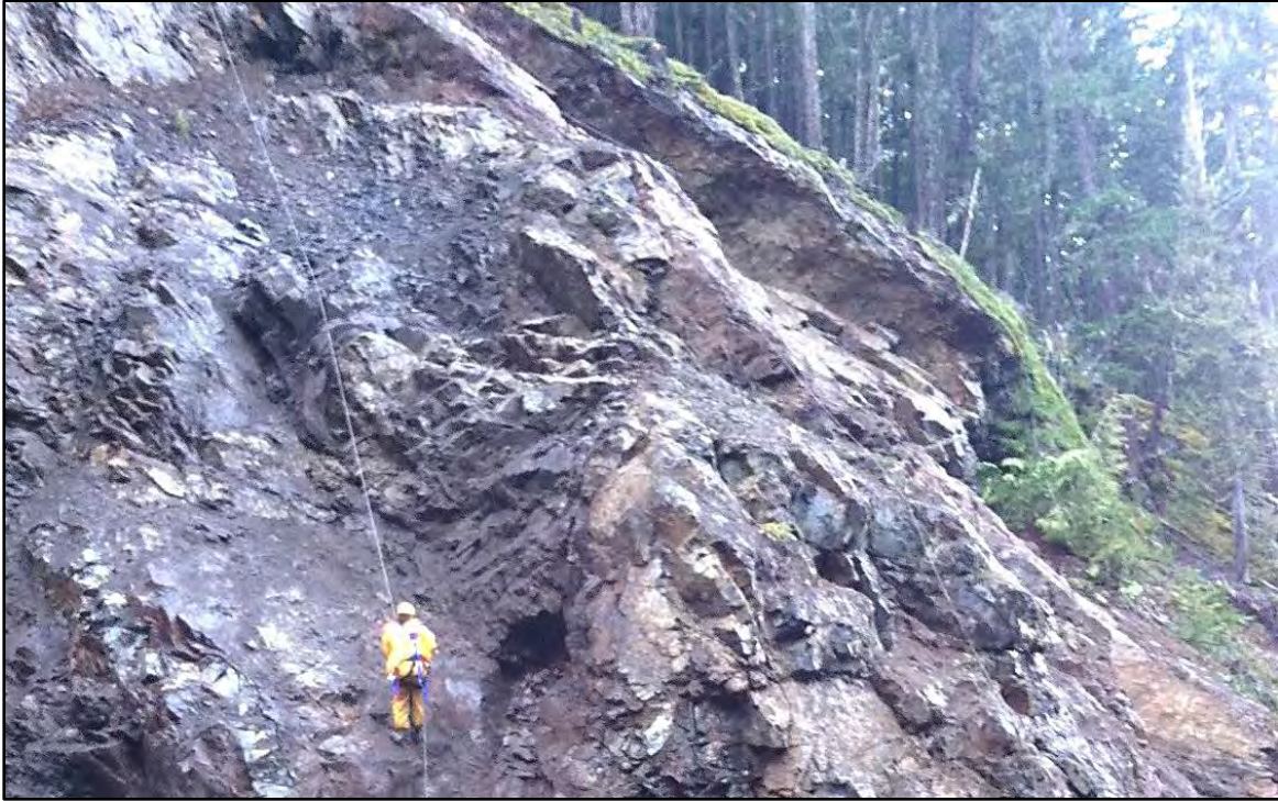
Figure 7: Collecting discontinuity measurements while rappelling on the slope.
