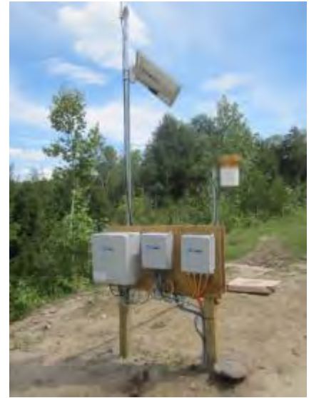
Figure 15 - Remote data collection and cellular communication system with solar panel power source.
