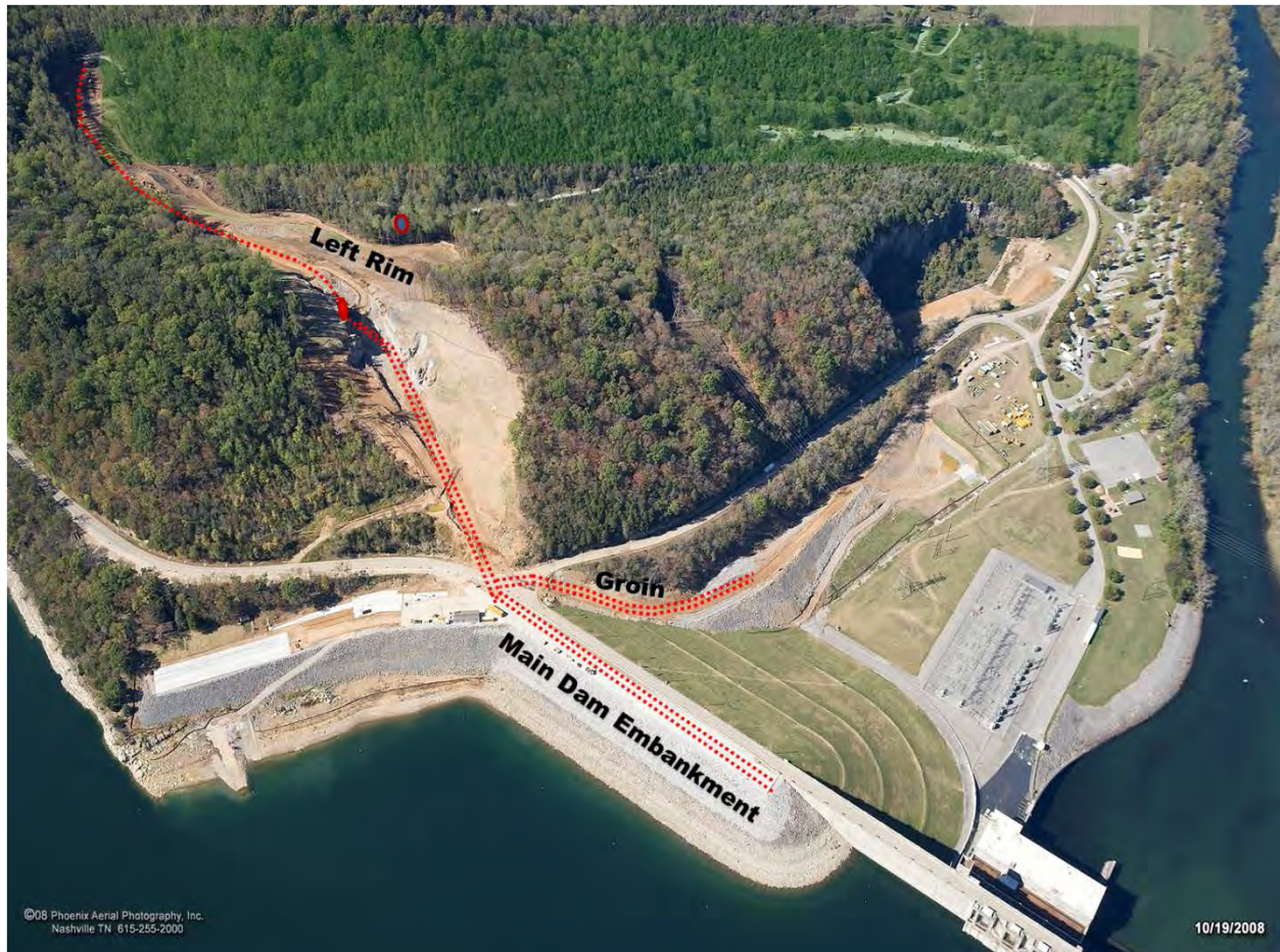
Figure 10. Aerial Photograph of Center Hill Site illustrating Grout Curtain Installation from 2009-2010.
