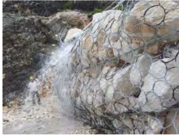
Figure 16 – Lateral view of the flexible debris flow barrier impacted during the full scale test carried out by the University of Parma in cooperation with Maccaferri
