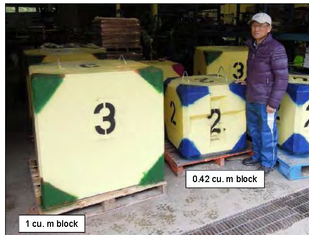
Figure 8: Concrete Test Blocks before testing.
