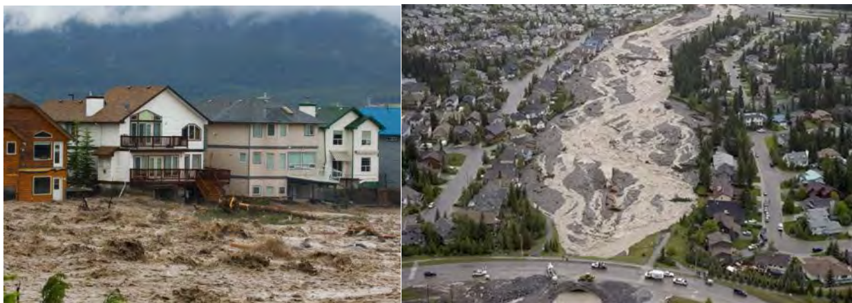
Figure 2 - Flooding on Cougar Creek threatened many residences (left) and channel aggradation lead to a braided river that caused significant bank erosion near Elk Run Boulevard (right). Town of Canmore.
