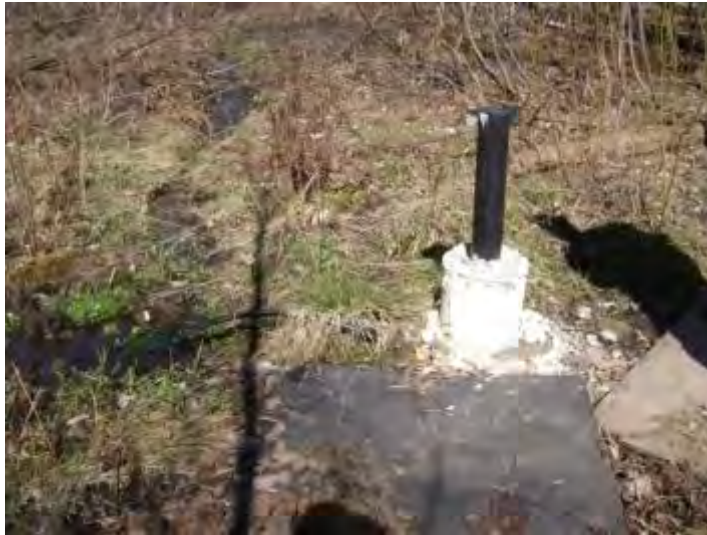
Figure 6 - Inclinometer near landslide toe installed in 1989 with artesian groundwater flow through pressure relief tube (~800 mL/min) (March 22, 2012).
