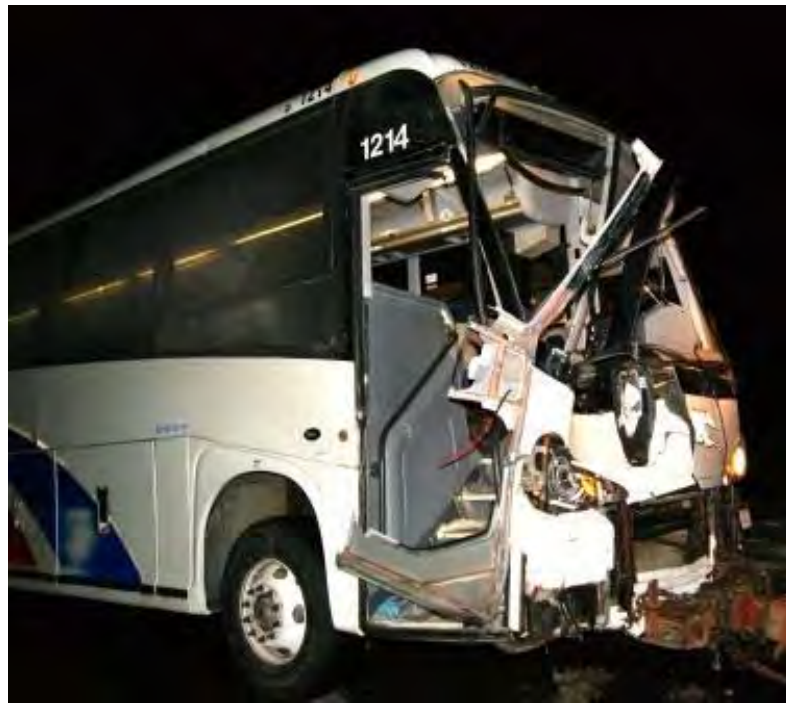
Figure 3 – Icefall impact to tour bus outside Terrace, British Columbia. Photo from Terrace Standard, 15 February 2011.
