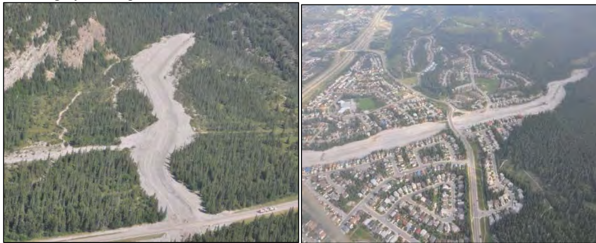
Figure 6. Comparison of roads crossing an undeveloped fan (left) and the highly-developed Cougar Creek fan (right) in Bow River Valley. Current practice would call for the same conveyance capacity design at each fan. BGC Engineering.
