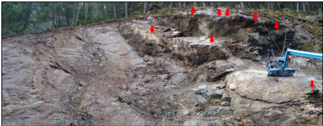
Figure 17: The red dots were monitored for movement every 15 minutes with a total station.
