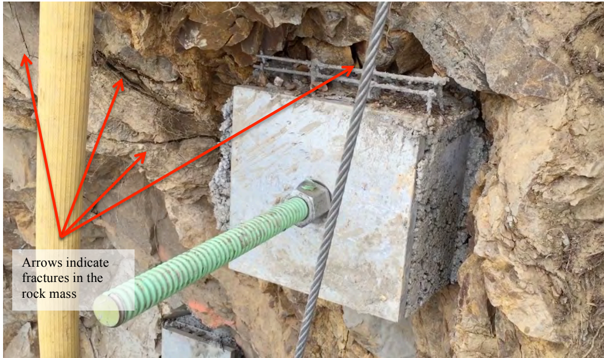
Figure 6 – Image of a rock anchor and surrounding rock mass after testing. Application of the test load fractured the rock mass and caused the rock anchor incapable of carrying the designed load.
