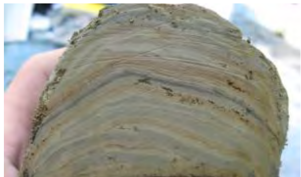
Figure 16 - Clay and silt varves exposed in sonic core sample.
