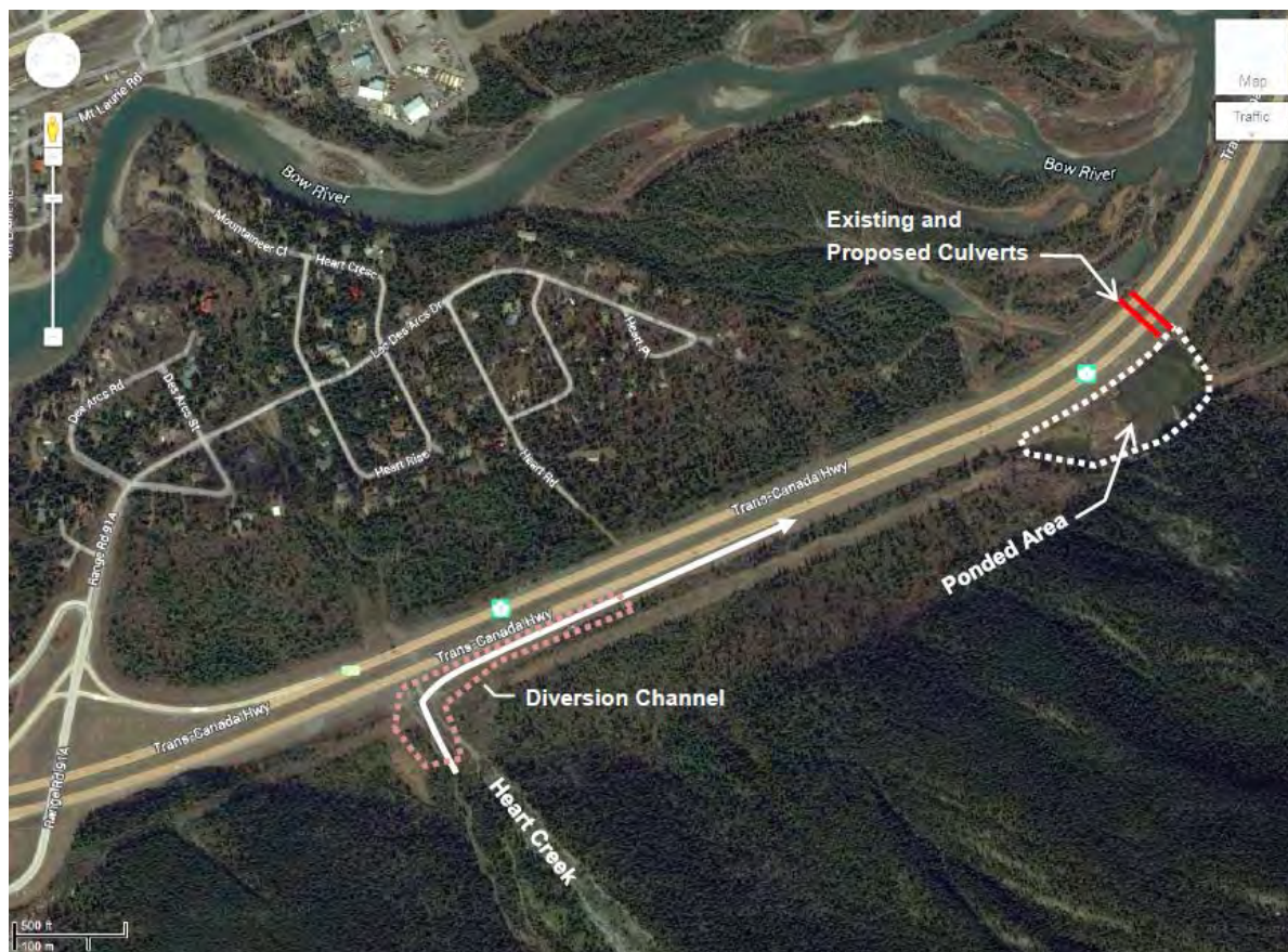
Figure 8 - Proposed Heart Creek debris-flood mitigation design. Google Earth.
