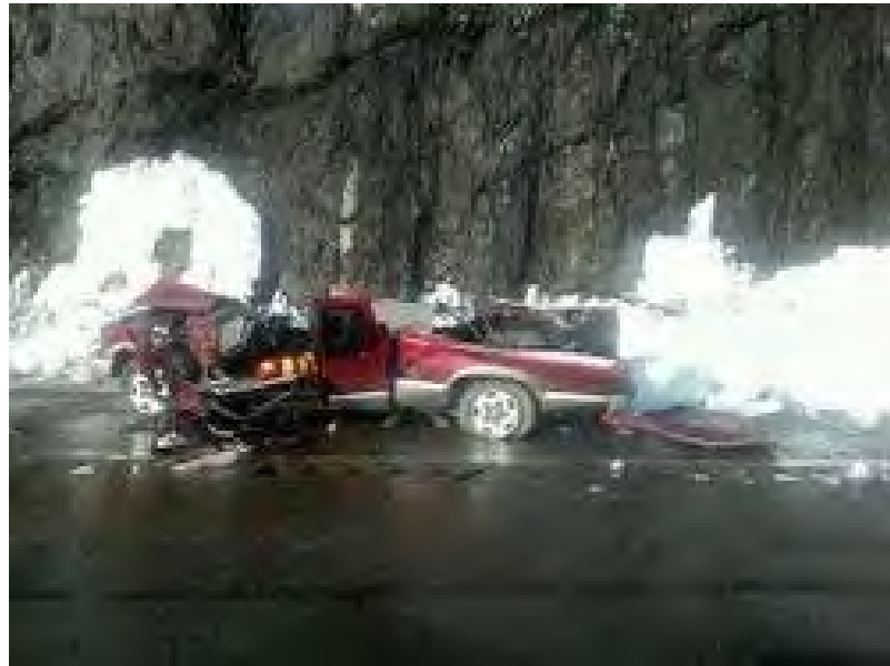
Figure 1 – Direct icefall impact damage to small pick-up truck along Seward Highway near Anchorage, Alaska. Photo courtesy of Anchorage Daily News, 6 April, 2012.
