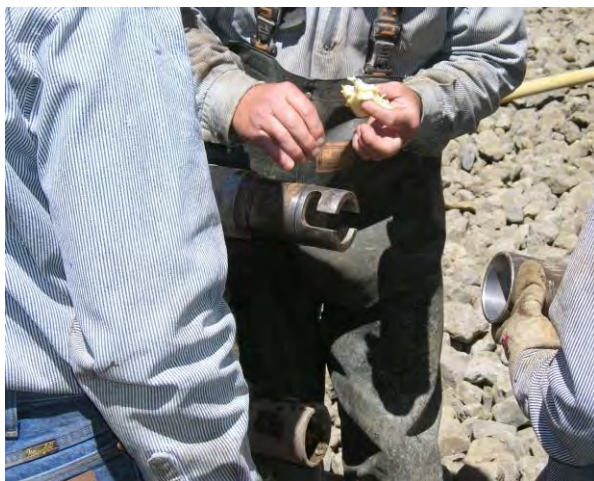
Figure 8 - View of "knock off" bit assembly.
