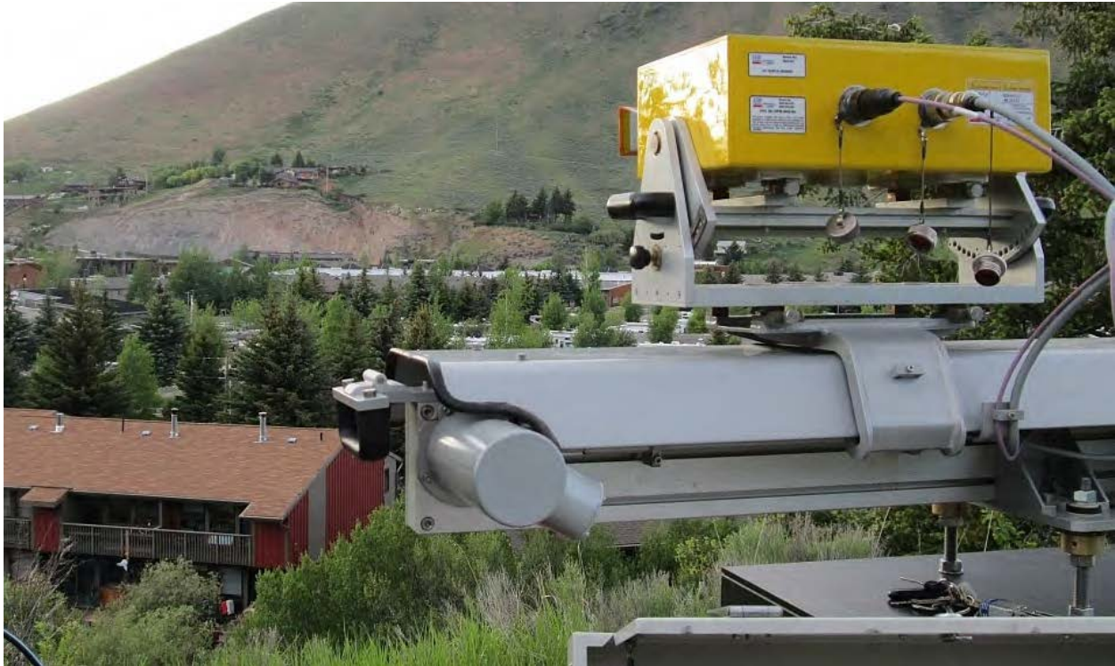
Figure 1: IBIS Interferometric Radar at the Karns Residence Facing the Budge Slide, May, 2014.
