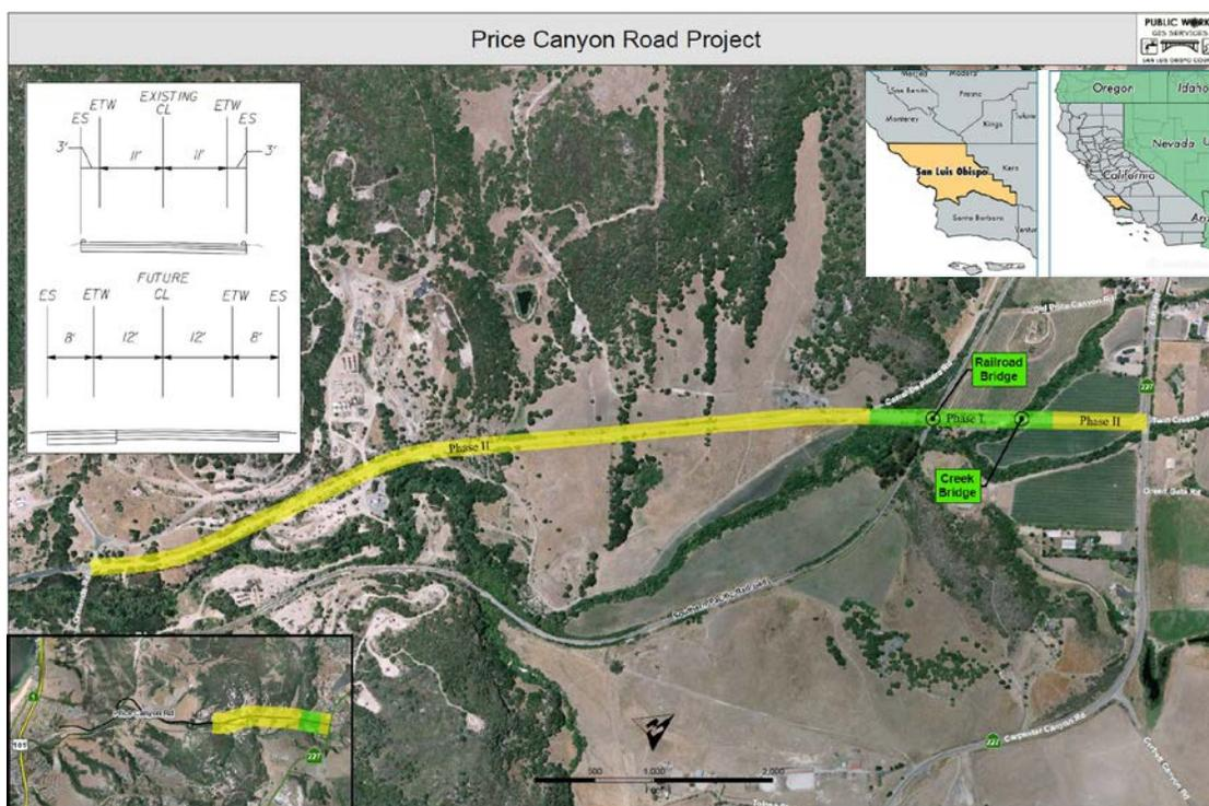
**Figure 1. Price Canyon Road Widening (Phase 2 Alignment in Yellow)**
