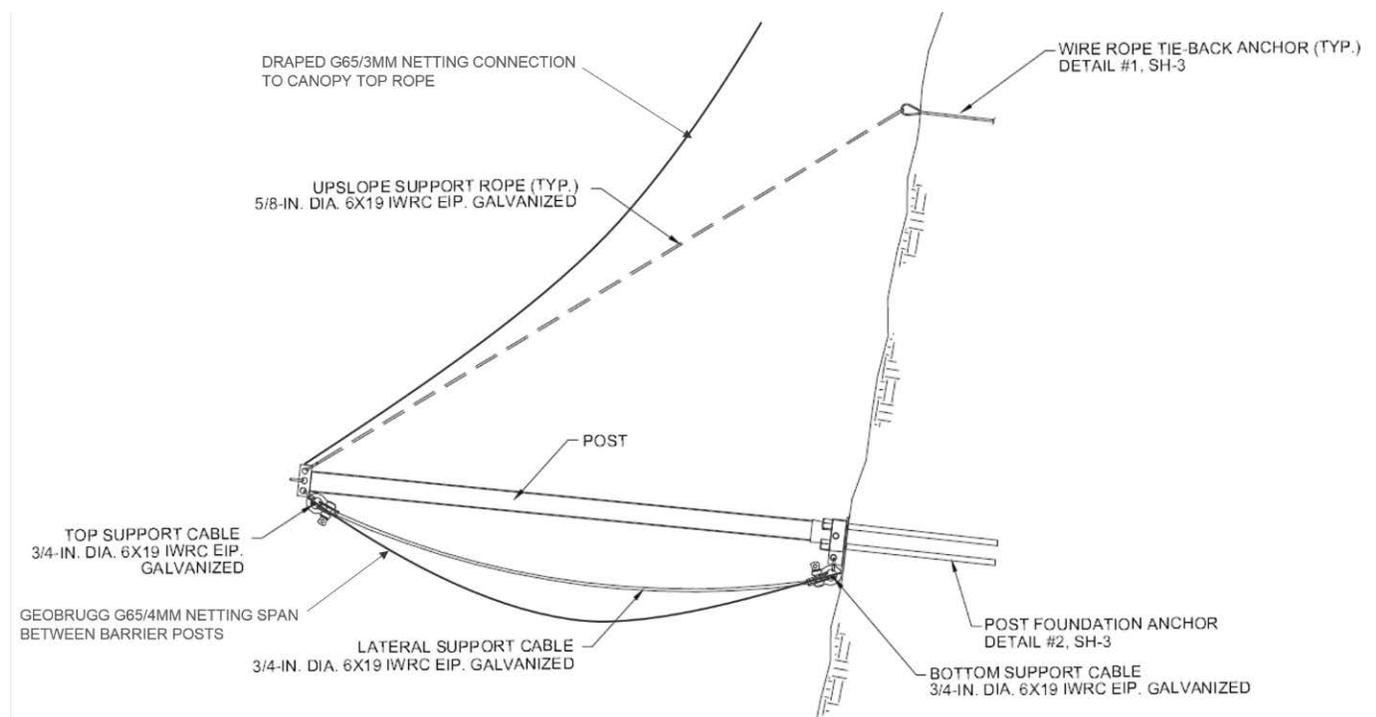
**Figure 4 – Canopy post section detail**
