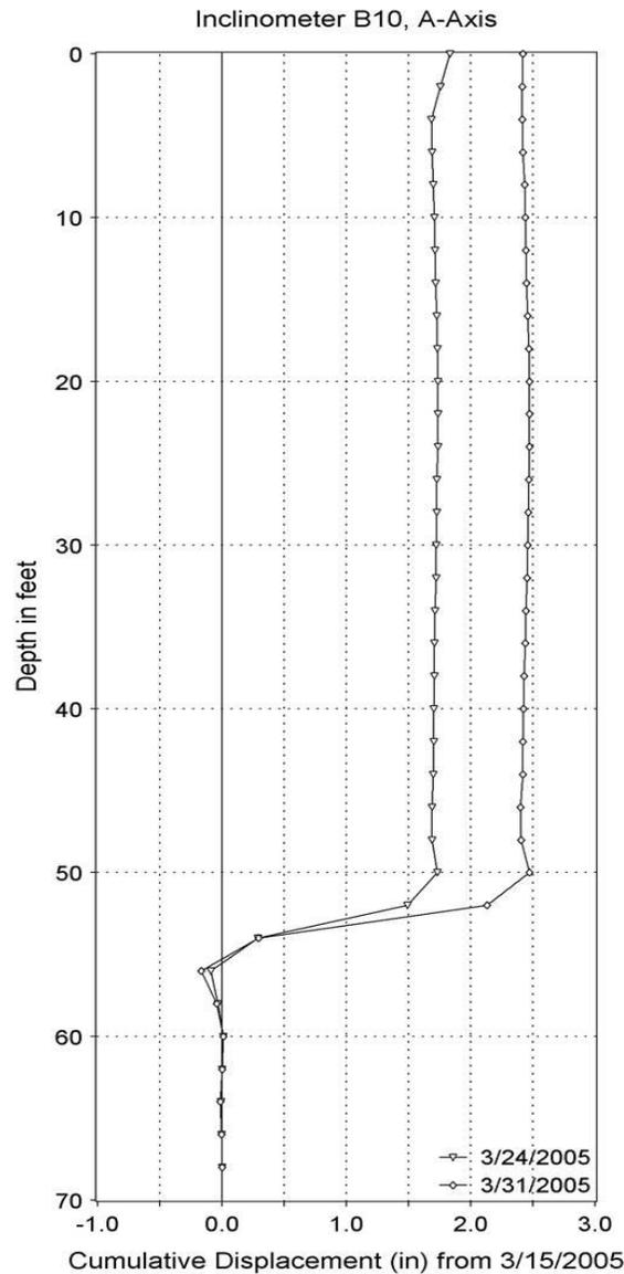
**FIG. 2 - Typical inclinometer results showing horizontal displacement before construction.**
