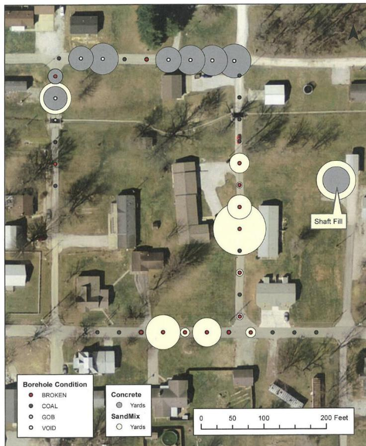
**Figure 7. Borehole Condition, Concrete and Sand Mix Footprints at Site 2146 Linton Grouting.**
