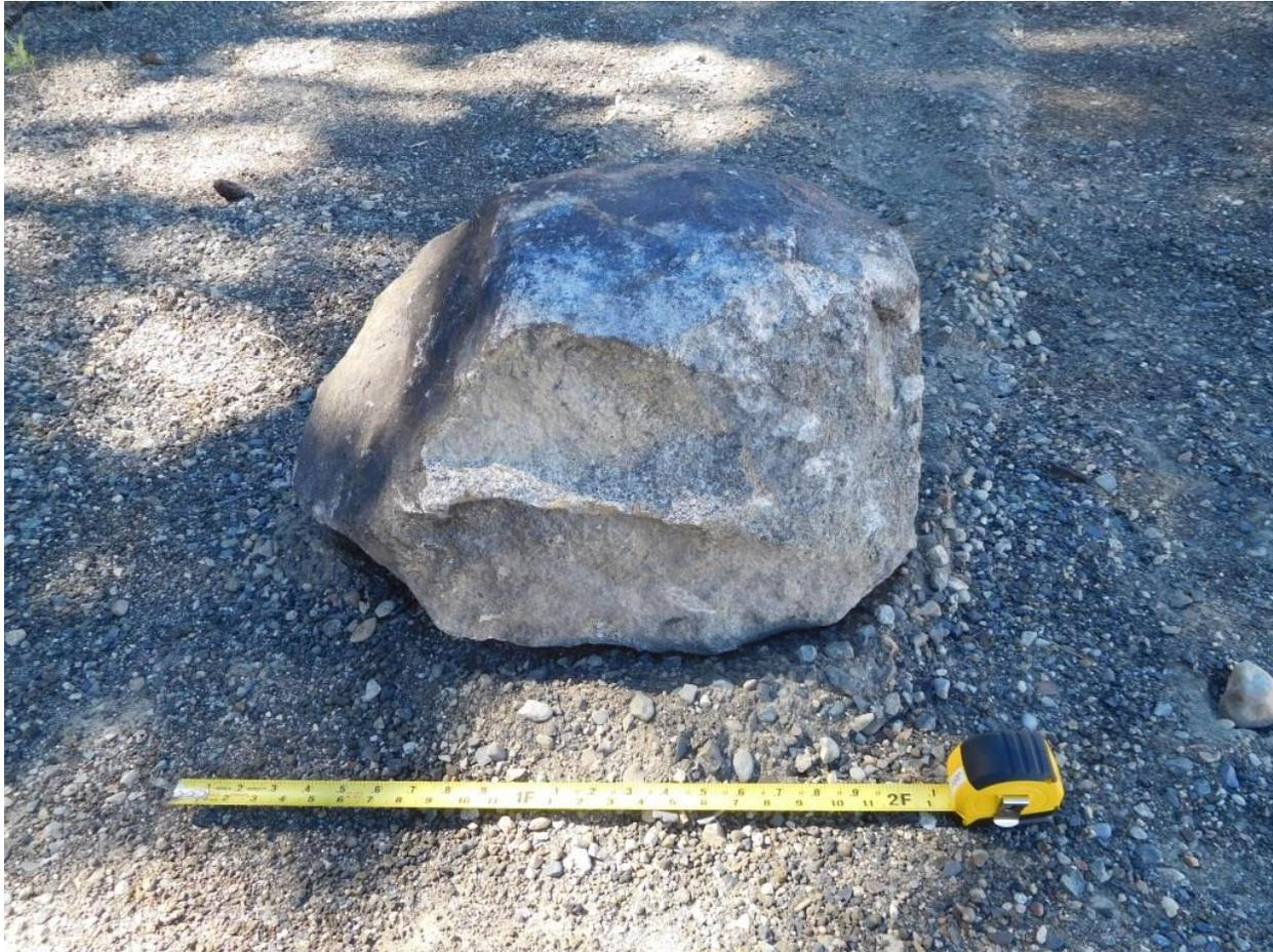
Figure 5. Largest rockfall observed in catchment area during field investigation on July 19, 2016.
