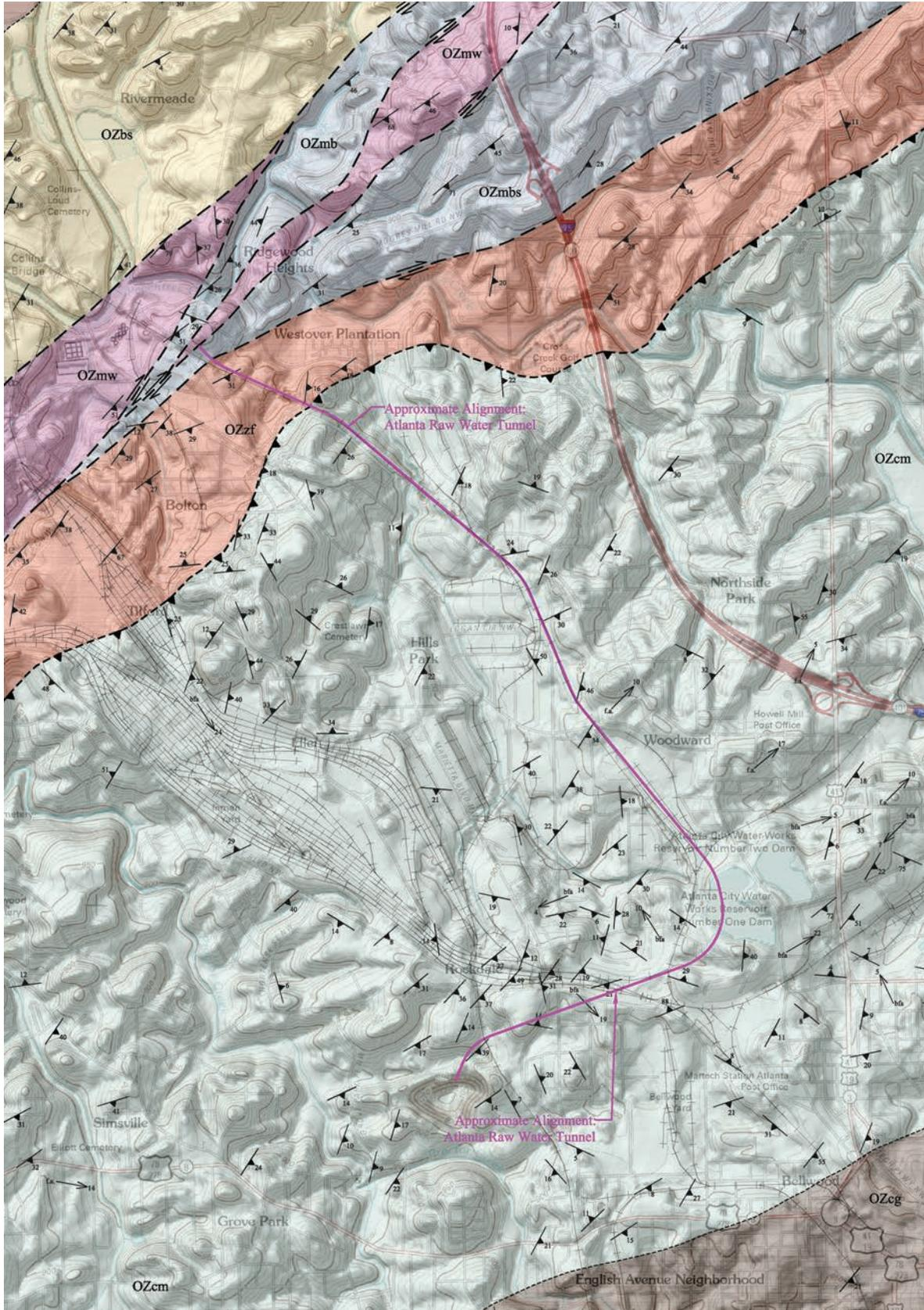
Figure 3. Detailed geologic map along the RWT alignment. See text for characteristics of each rock unit. OZbs- button schist, OZmw- Brevard Zone white mylonites, OZmb- Brevard Zone black mylonites, OZmbs- Brevard Zone black mylonites and button schist, OZzf- zoned feldspar gneiss, OZcm- Clairmont Mélange, OZcg- Clairmont Mélange gneiss.
