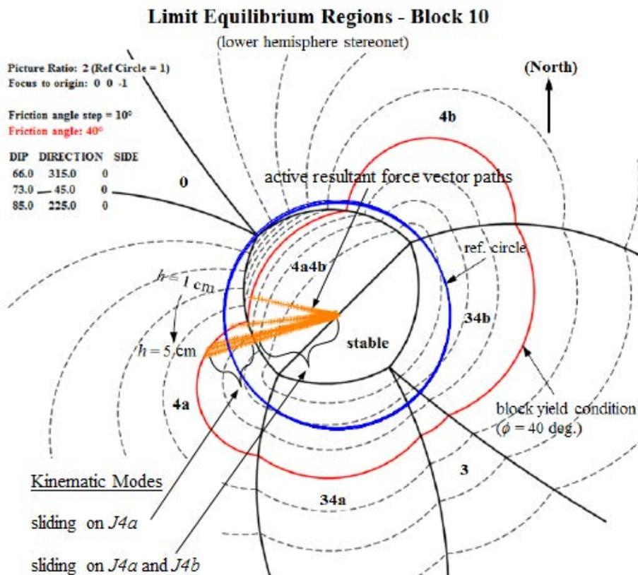
**Figure 2 – Limit equilibrium stereonet showing change in block kinematic failure mode in response to external loading (adapted from George 2015)**
