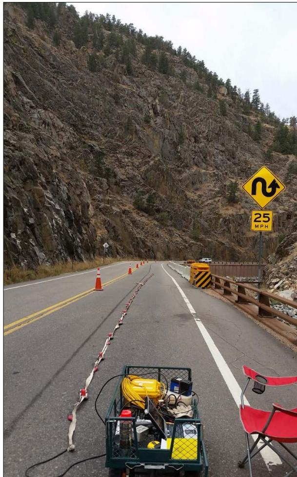
**Figure 6. Photograph of the seismic survey deploying the ‘landstreamer’.**
