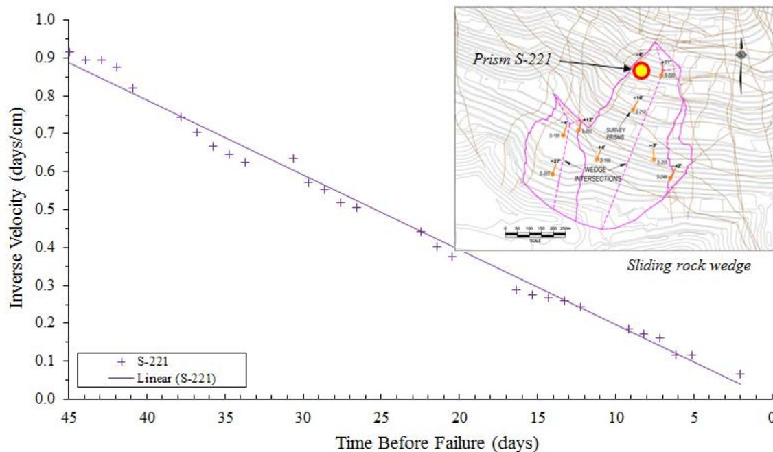
**Figure 6 – Inverse velocity time series for rock wedge leading up to failure for Barrick Gold's Betze-Post open pit mine (adapted from Rose & Hungr 2007).**
