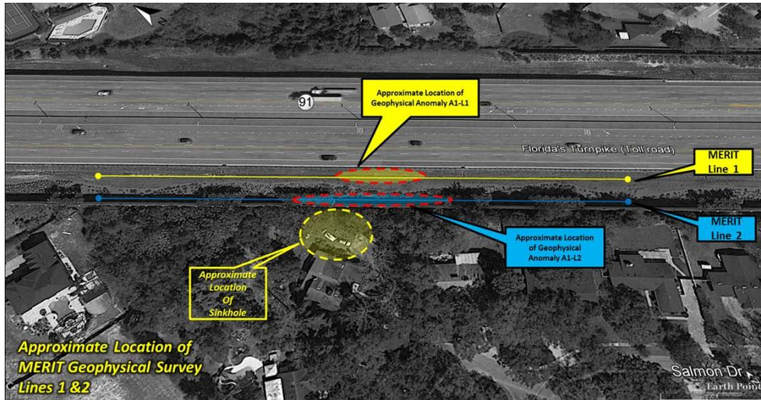
**Figure 2: Image of the MERIT Lines, sinkhole and anomalies**
