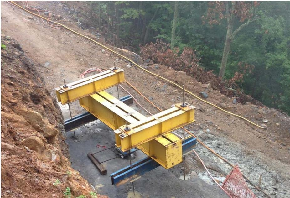
**Figure 9 – Compression Load Test Setup**
