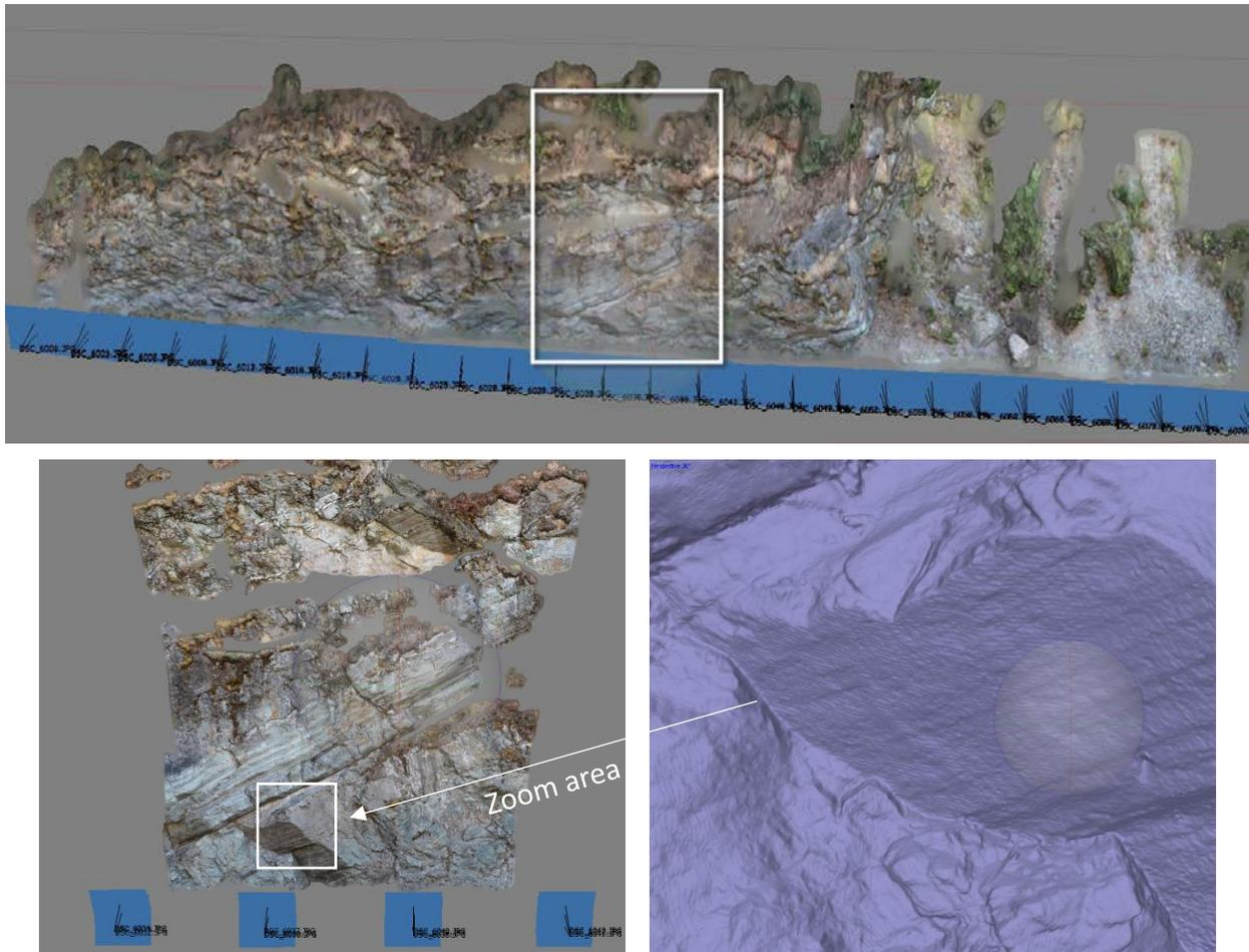
**Figure 2: US 2 Badrock Canyon Model. Photo model on the left and a detailed solid model on the right, zoomed in from the upper photo model at the top.**
