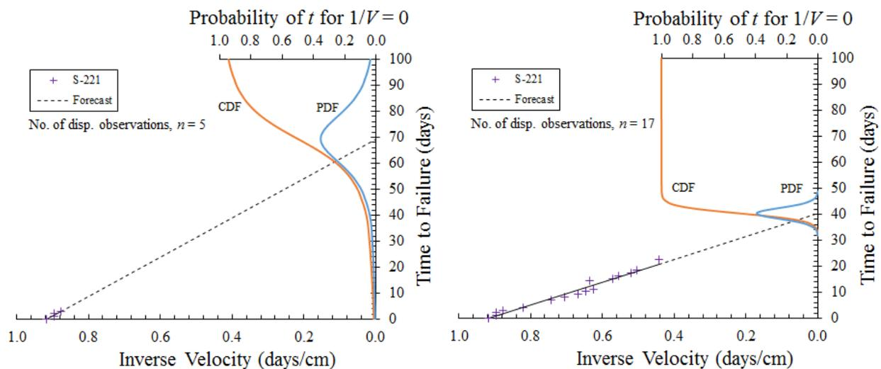
**Figure 7 – PDF and CDF for time to failure forecast given  $n = 5$  observations (left) and  $n = 17$  observations (right) assuming  $1/V = 0$ .**
