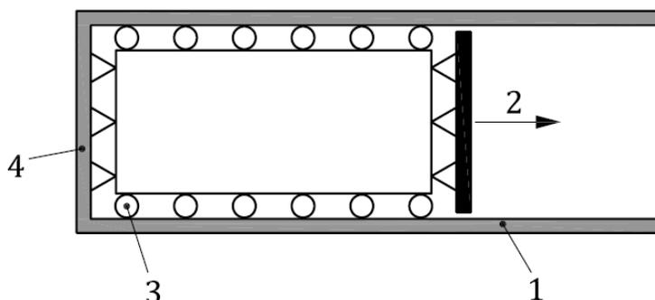
**Figure 3** - Example of frame configuration for the tensile strength test. Legend: 1) Fixed frame; 2) Movable beam; 3) Lateral constraint; 4) Side connection device.
