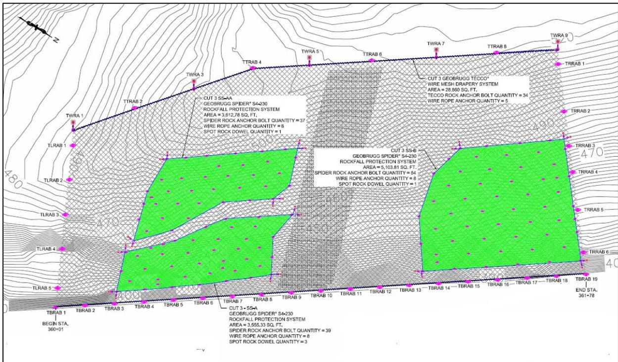
8. Final plan for Northern highwall using tensioned Spider mesh overlaid with TECCO drapery
