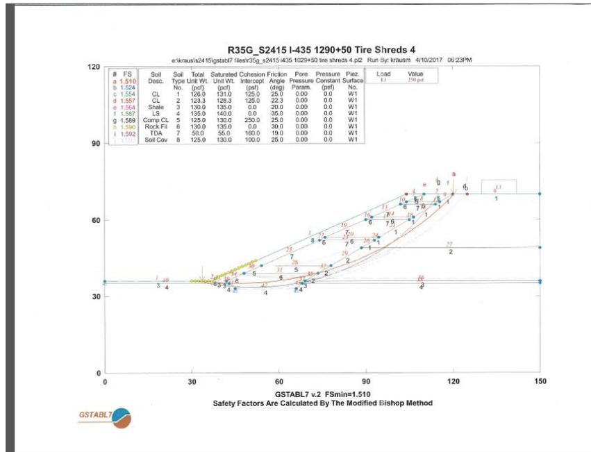
Figure 5 – TDA Slope Analysis With Lower Soil Layer
