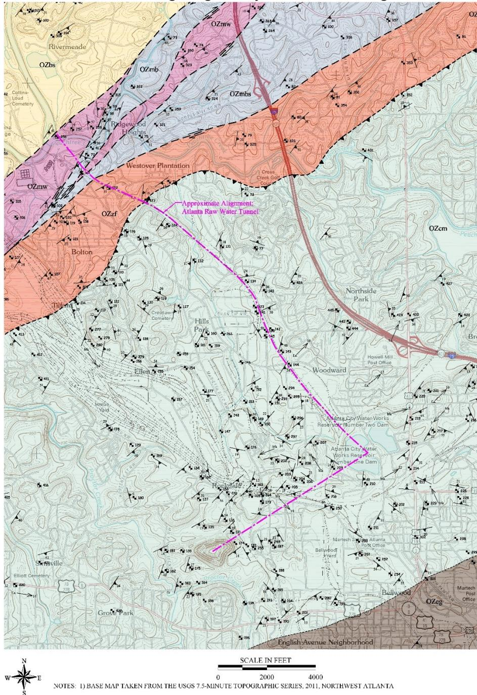
Figure 5. Geologic map prepared during the initial field mapping for the Water Supply Program tunnel project.
