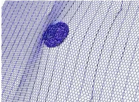
**Figure 2** - Numerical model of Mesh restrained by means of 4 anchor plates.
