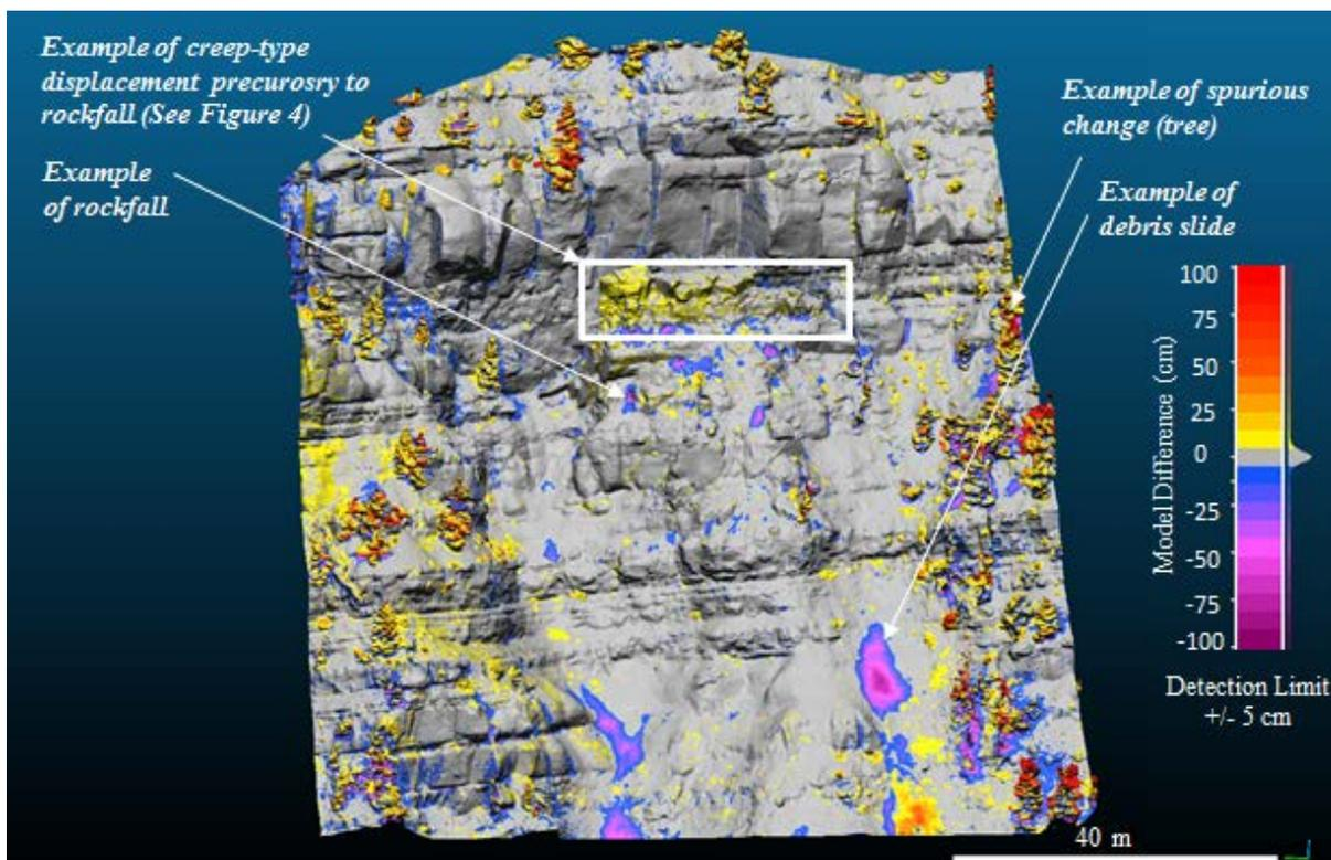
**Figure 3 – OAP change detection map and examples of rockfall, precursory rockfall displacement, debris slide, and spurious change (adapted from Christiansen et al. 2016).**
