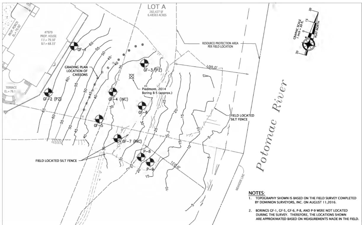
**Figure 1: Boring Location Plan**
