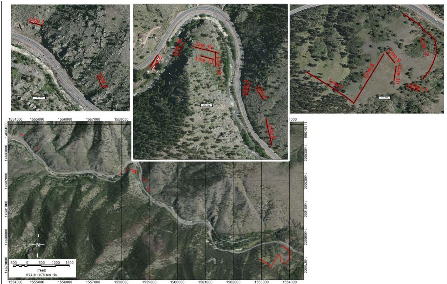
**Figure 11. Line location map from first seismic survey, showing 16 separate line positions.**
