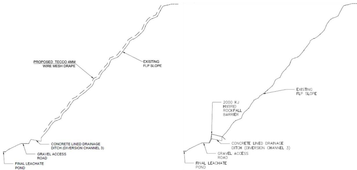
**Figures 7A (left) – Drape design section, and 7B (right) – Hybrid rockfall barrier design.**
