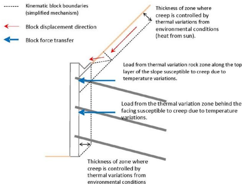
**Figure 7. Rock Dowel Wall Surficial Loading Mechanisms**
