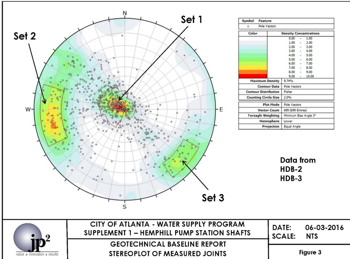
Figure 9. Stereoplot from the Geotechnical Baseline Report of geophysical information showing the high angle joint sets.
