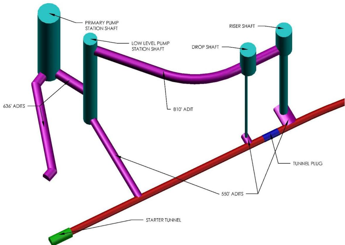
**Figure 3. Arrangement of the structures at the quarry site.**
