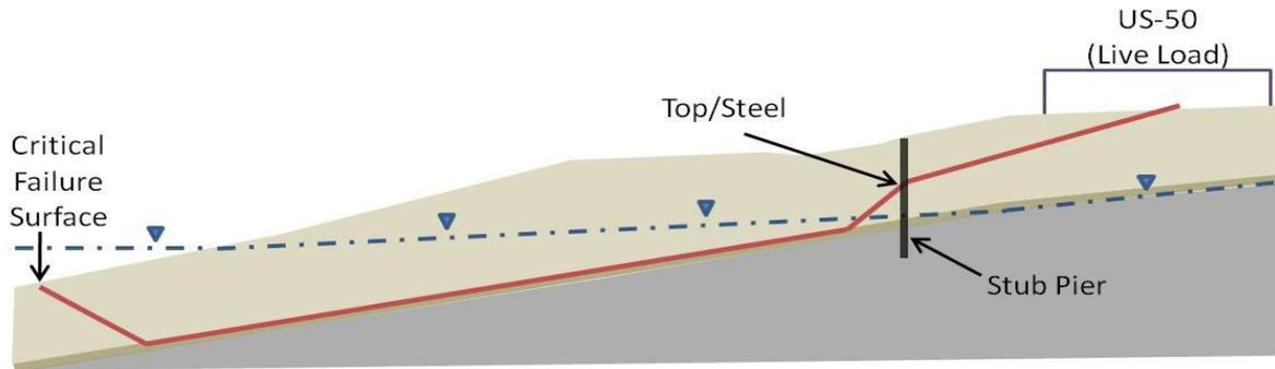
**FIG. 2 - Slope stability schematic.**
