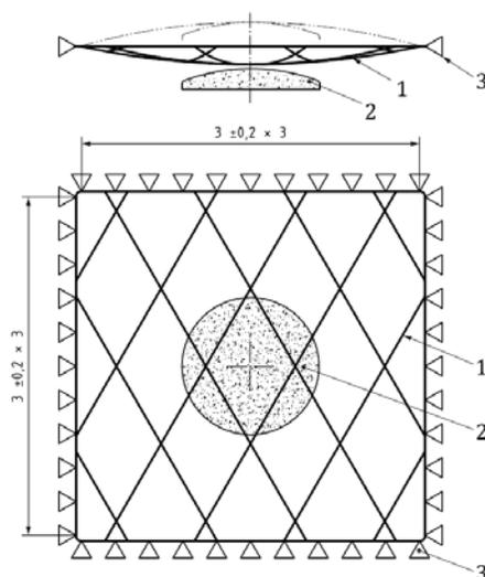
**Figure 4** - Example of set up for punching test according to ISO 17745 and ISO 17746. Legend: 1) Tested mesh sample; 2) hemispherical shaped load sharing device (1.0 m in diameter); 3) Perimeter constraint between the mesh and the frame.
