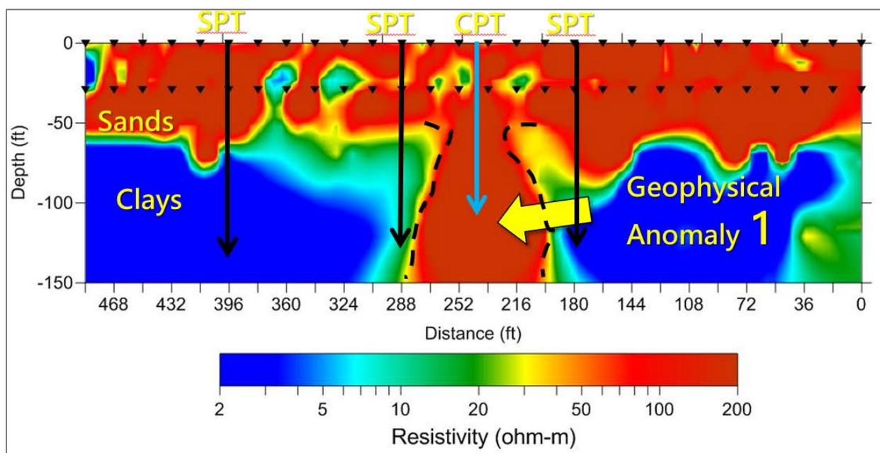
**Figure 4: Results of MERIT Line 1 and location of geotechnical testing**
