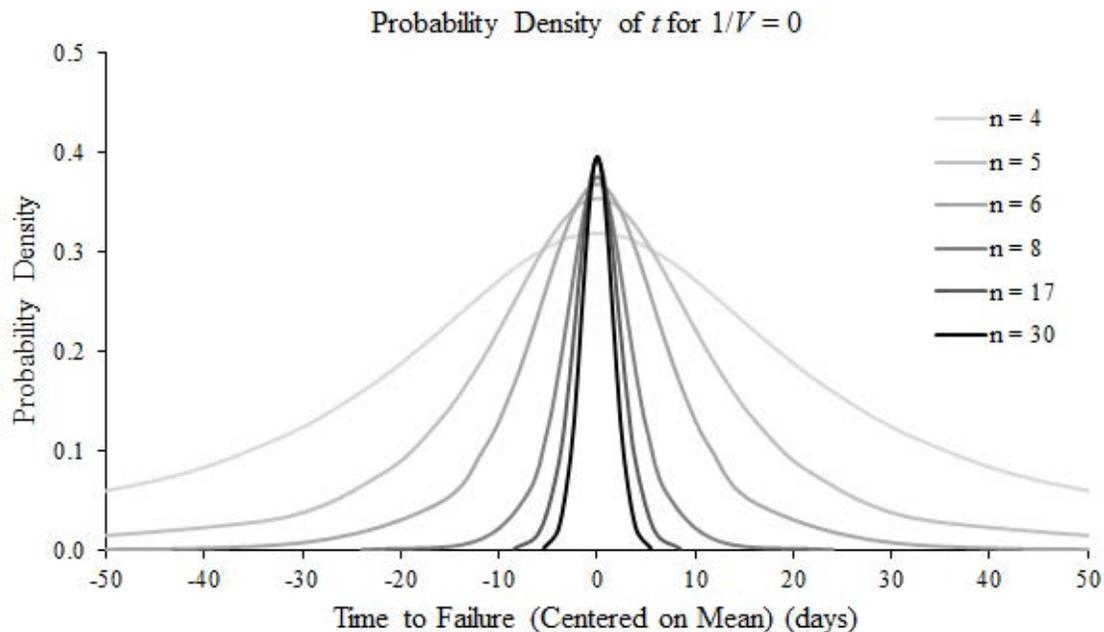
**Figure 8 – Progression of posterior predictive PDF for time to failure forecast with increasing number of observations.**
