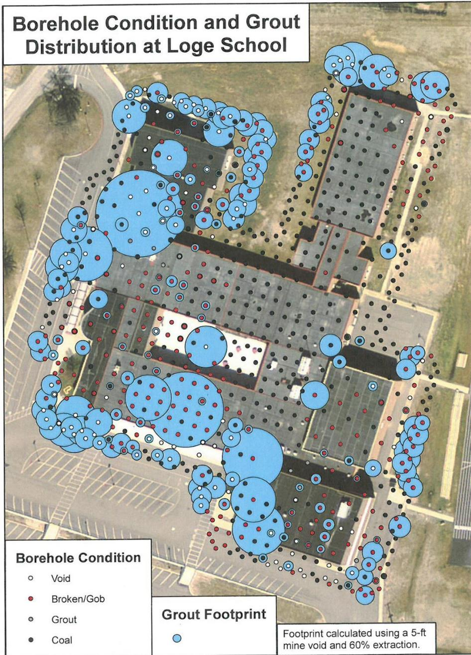
**Figure 6. Borehole Condition and Grout Distribution at Loge School**
