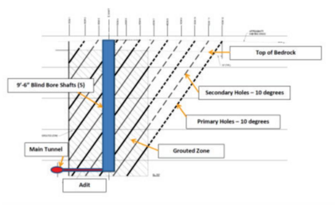
Figure 8. Cross-section view of the pre-excitation grout holes.
