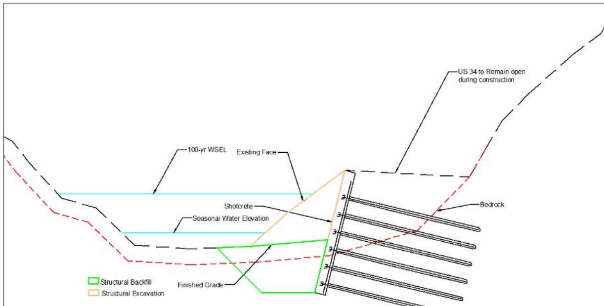
**Figure 5. Schematic of potential scour resistant element design.**
