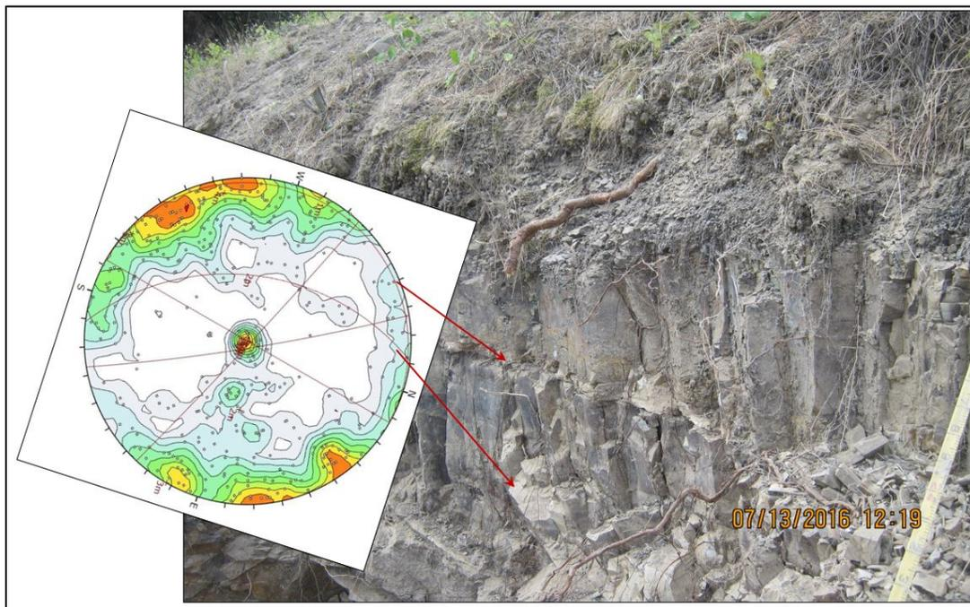
**Figure 10 – Joint Set 1 (bedding) and Joint Set 2.**
