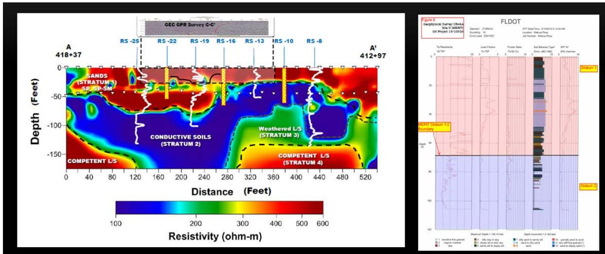
**Figure 3: Comparison of the geotechnical SPT and CPT results compared to MERIT**
