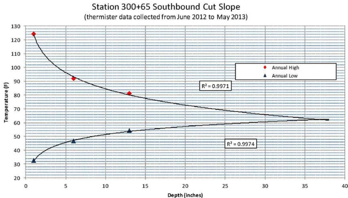
**Figure 6. Annual Temperature Extremes within Bituminous Sandstone**
