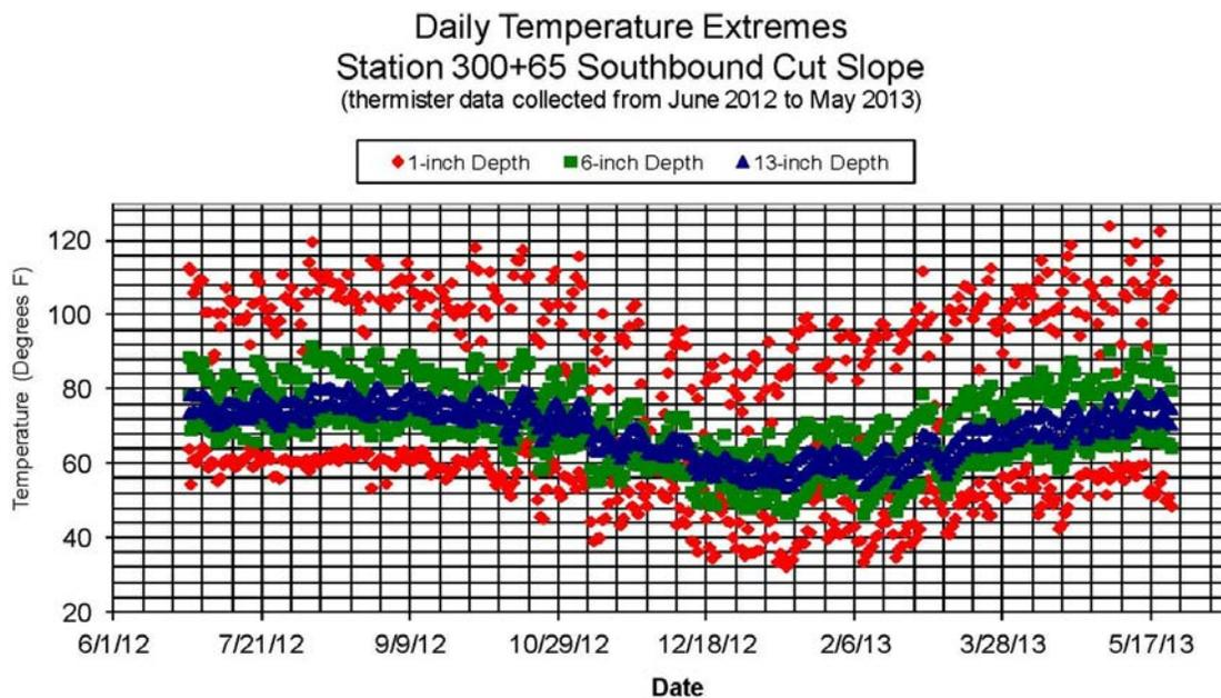
**Figure 5. Daily Temperature Extremes Within a Bituminous Sandstone Slope**
