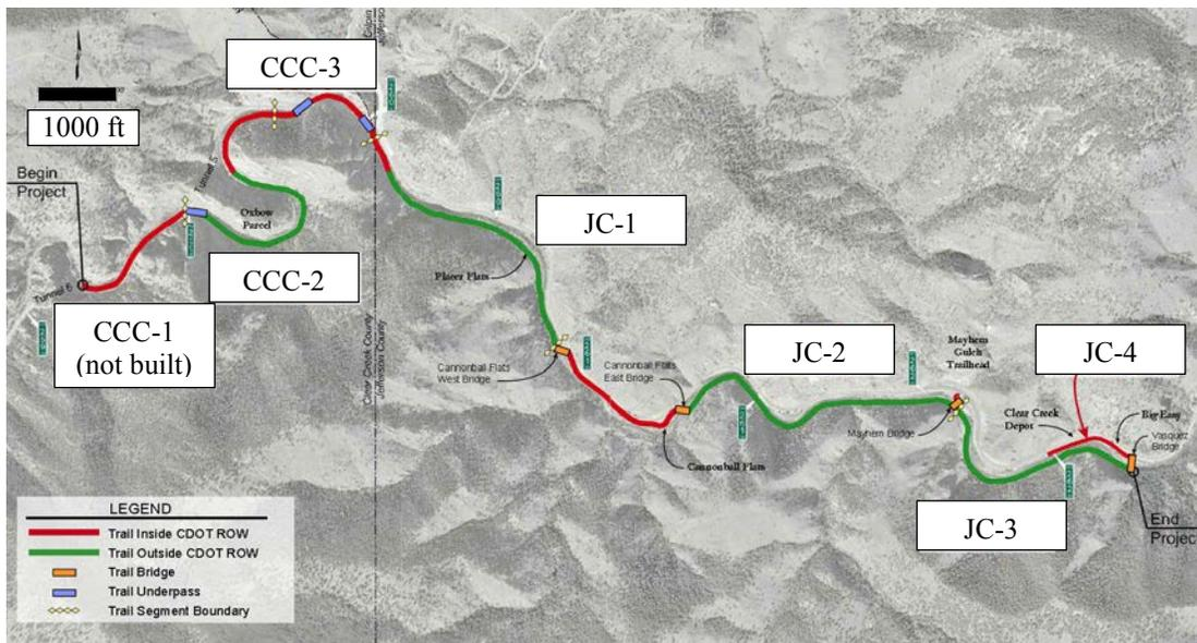
**Figure 2 – Project extents and construction segments (CC: Clear Creek County, JC: Jefferson County)**
