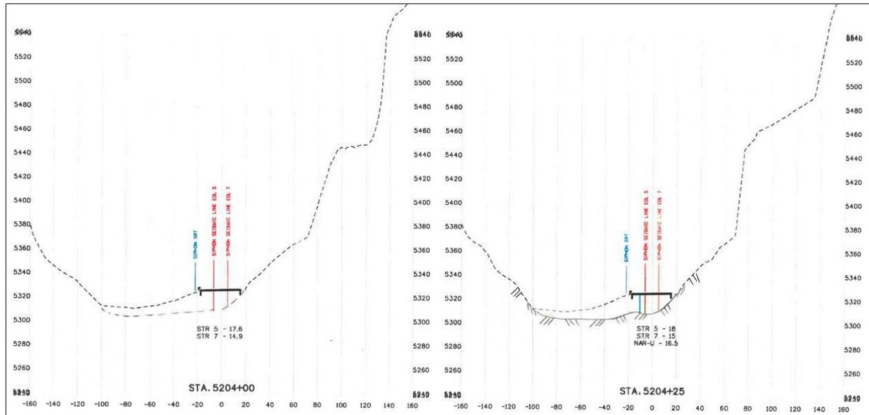
**Figure 10. Cross sections created with results from drilling (blue) and geophysical (red) investigations in The Narrows.**
