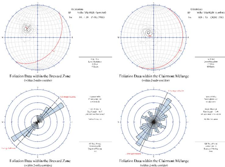
Figure 7b. Equal-area stereonet and rose diagrams of measured foliation from the Brevard Zone and Clairmont Mélange.
