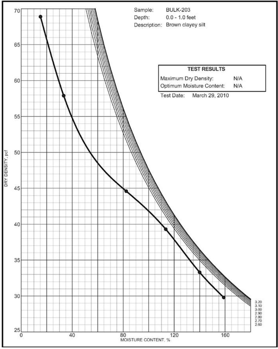
Figure 4 - Example Proctor test result from Saddle Road, East Side (21)
