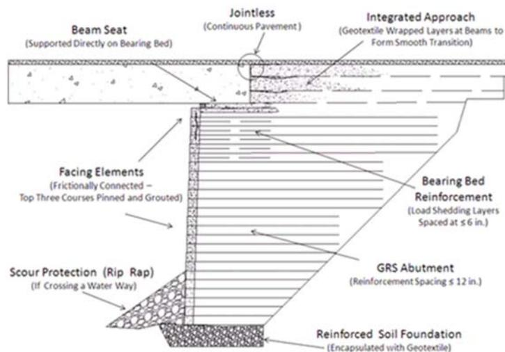
**Figure 19: Example truncated GCS wall (I)**
