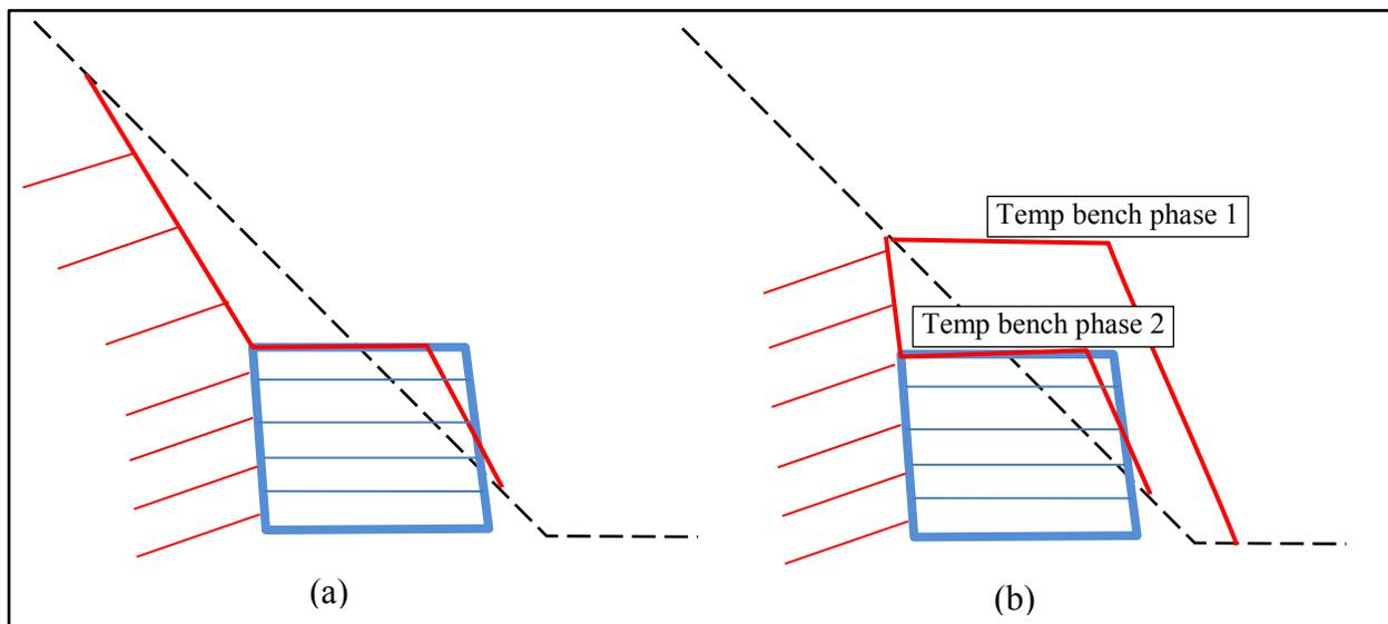
**Figure 10 – (a) Pioneering approach used for the project, requiring greater height of temporary shoring. (b) A different approach may have required less temporary shoring, but with other consequences.**
