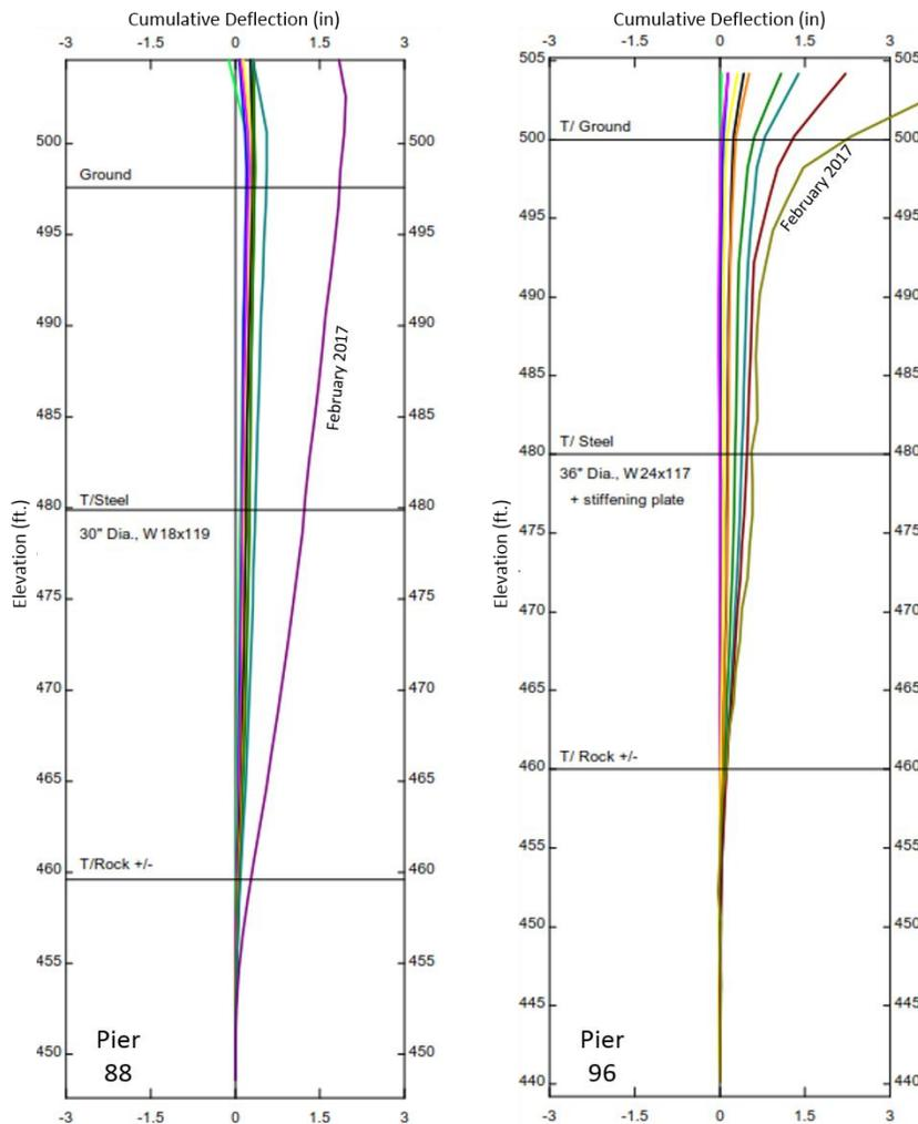
**Figure 4 – Inclinometer Readings at Piers 88 and 96, 2005 to 2017**
