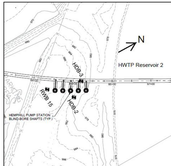
Figure 6. Site layout at Hemphill showing blind bore shafts and adits connecting to the main tunnel.
