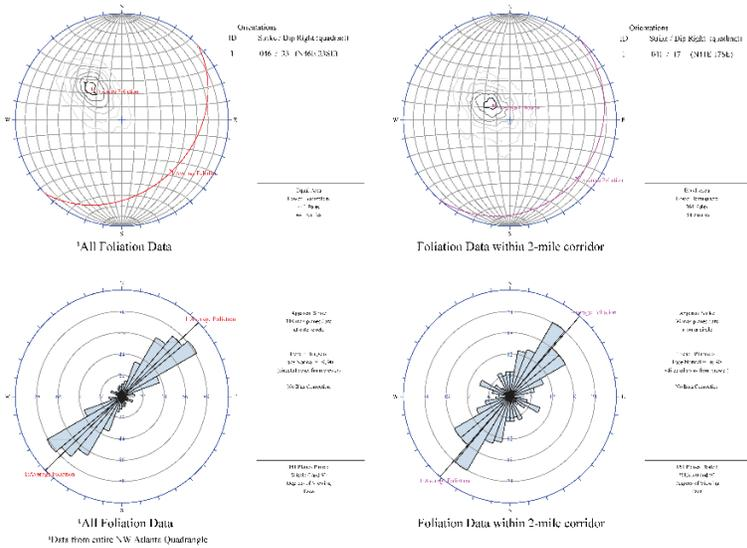
Figure 7a. Equal-area stereonet and rose diagrams of measured foliation from all mapping and measured foliation within a 2-mile corridor.
