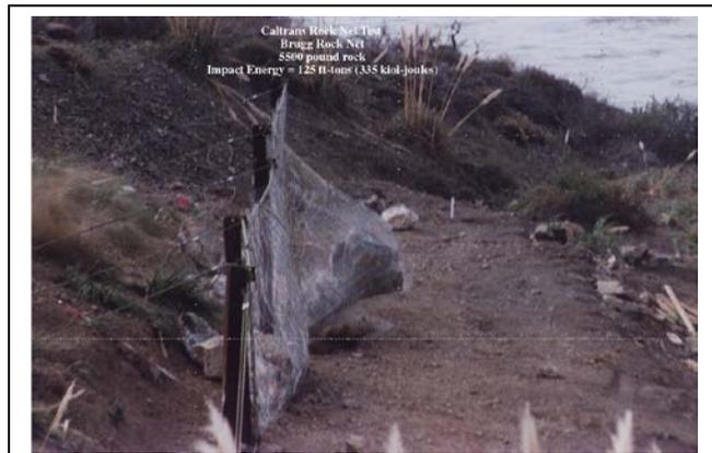
**Figure 7 – Early CalTrans Rockfall Barrier Testing**
