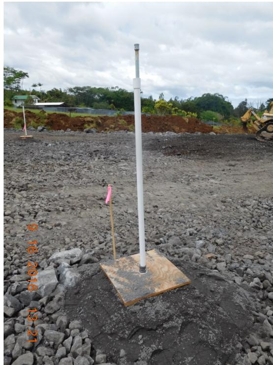
**Figure 10 - Typical settlement monitoring point assembly. Assembly was installed near the base of embankment to measure settlement of subgrade ash.**
