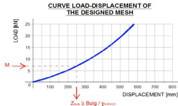
**Figure 7** - Example of a curve load-displacement used for the design of the mesh at the Serviceability Limit State.
