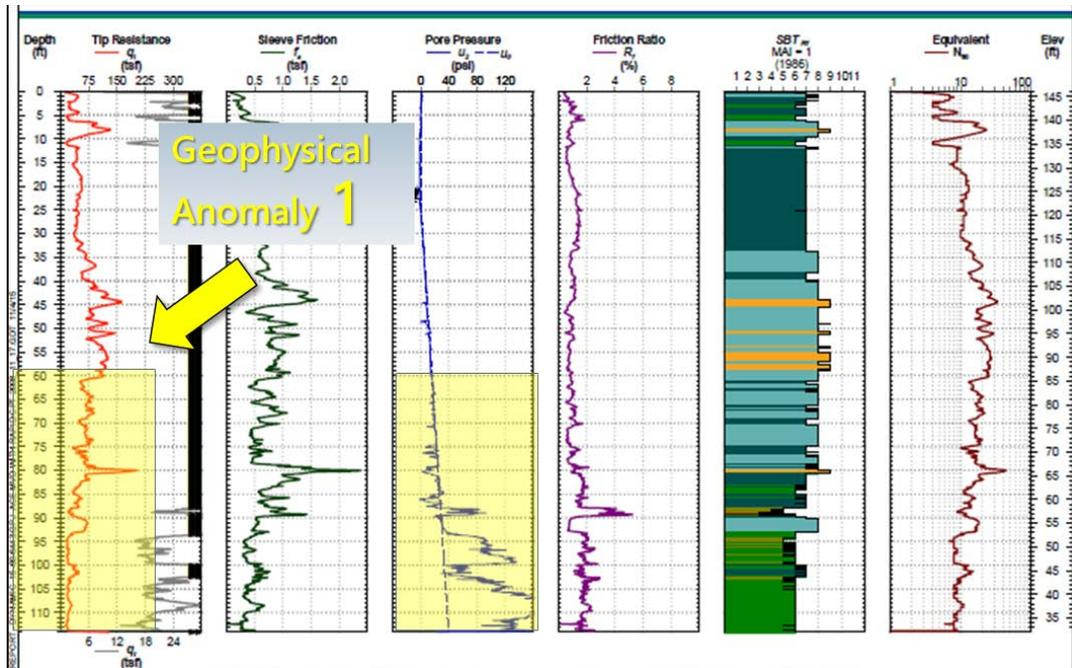
**Figure 5:** Results of CPT at the location of the geophysical anomaly Line 1
