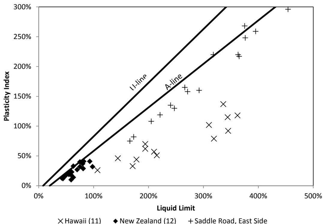
**Figure 1 - Casagrande classification of select weathered volcanic ash samples from Hawaii and New Zealand.**
