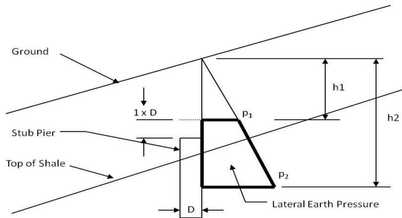
**FIG. 3 - Earth Pressure Schematic**
