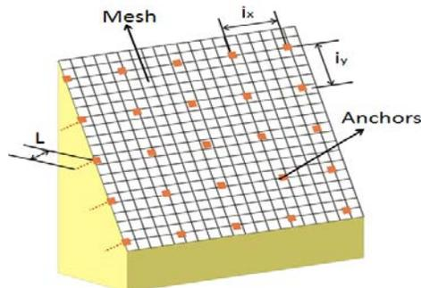
**Figure 1** - Pin drapery system: the intervention is composed by a rockfall mesh and a pattern of anchors ( $L$  = length of the anchors;  $i_x$  and  $i_y$  = distance between the anchors, respectively horizontally and vertically).
