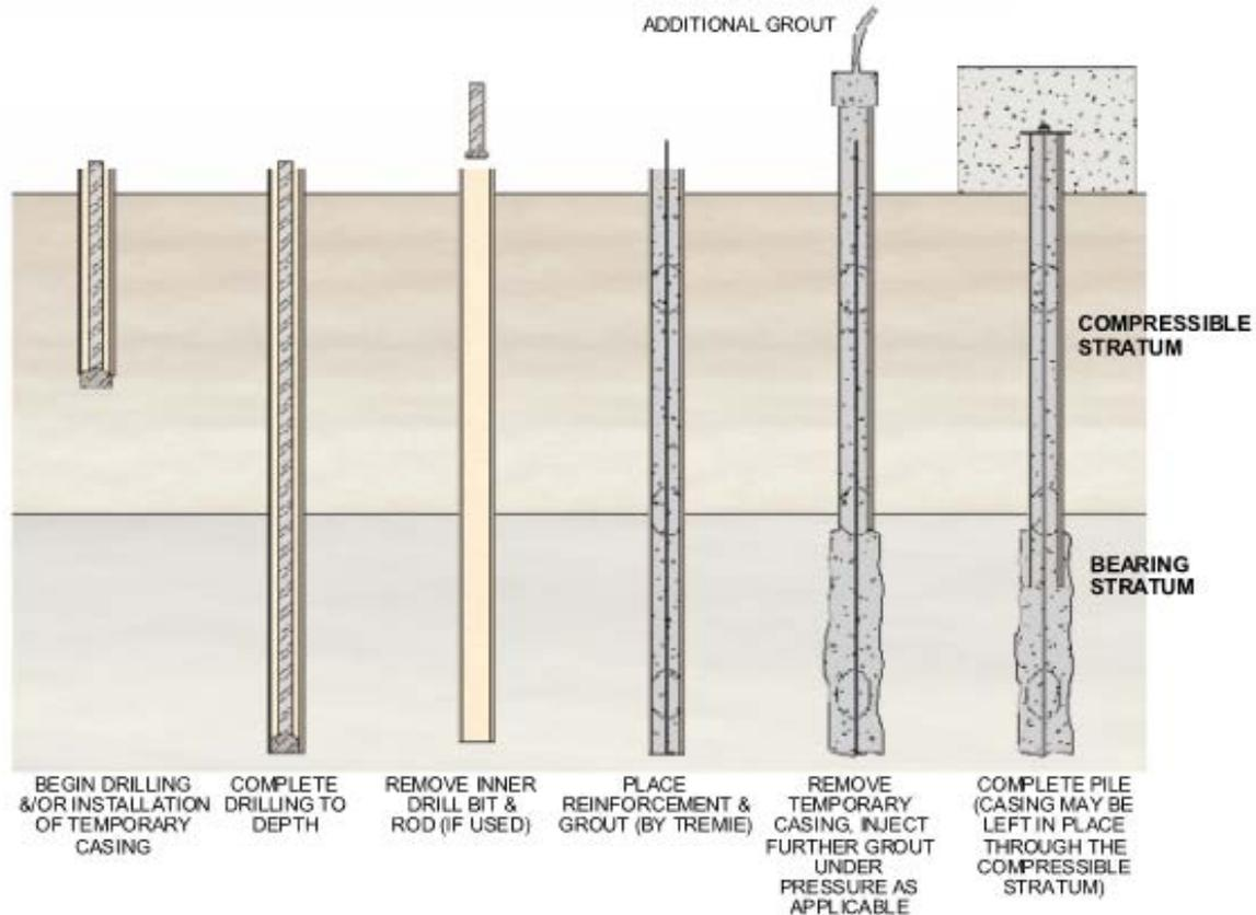
**Figure 4 – Micropile Installation (Sabatini et. al. 2005)**
