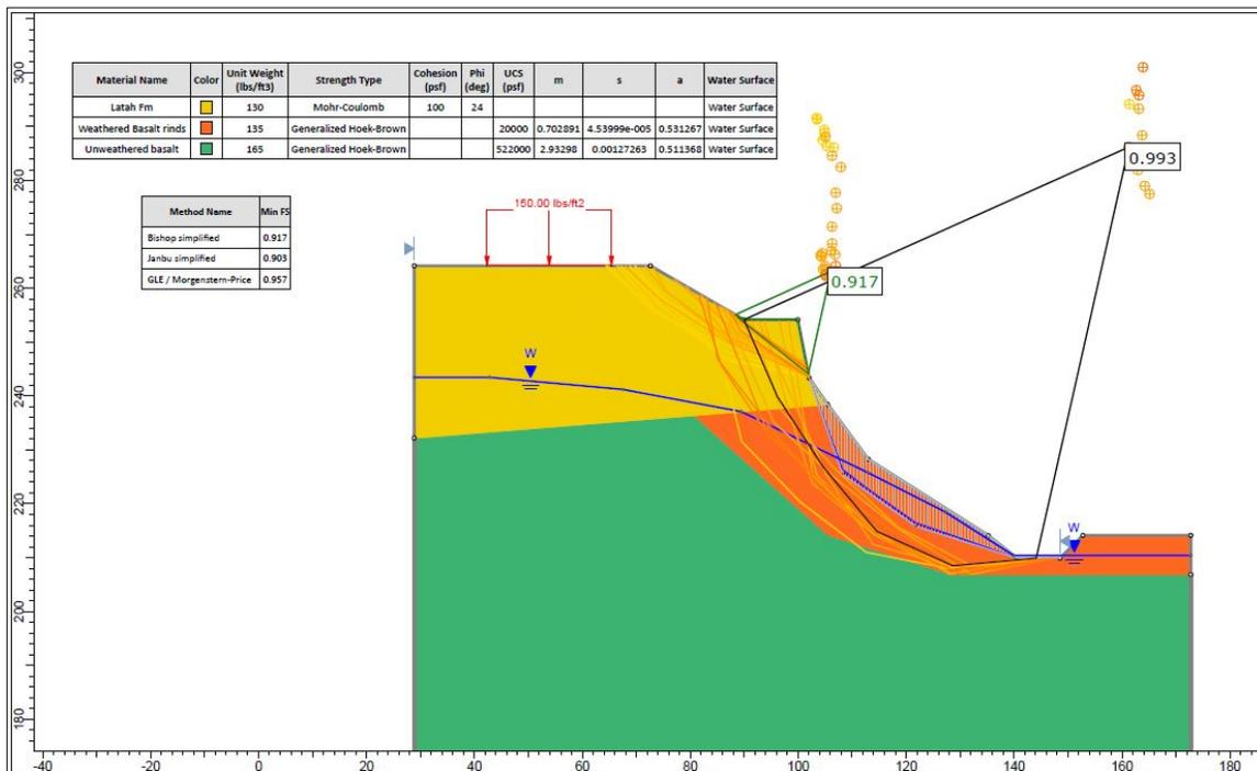
**Figure 11 – Base case Slide Model showing Latah (yellow), weathered (orange), and unweathered (green) basalt.**
