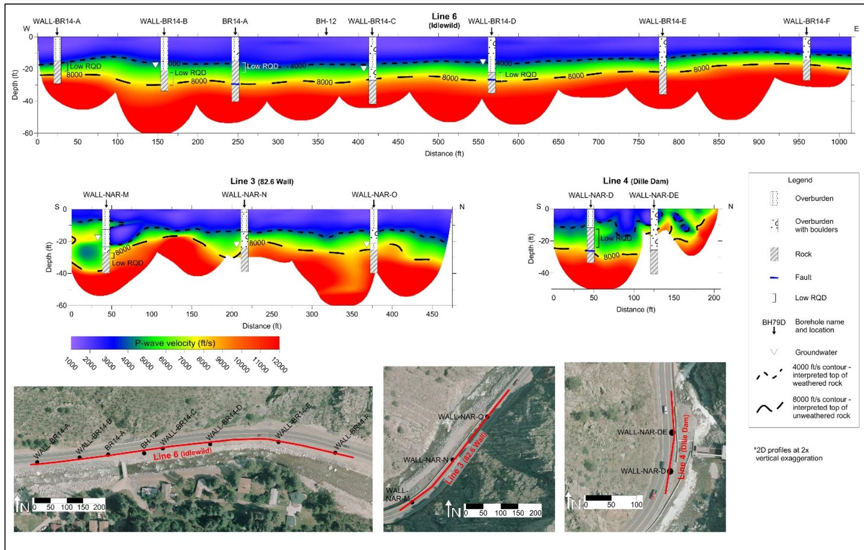
Figure 14. SRT Results from the second seismic investigation; Lines 6, 3, and 4.
