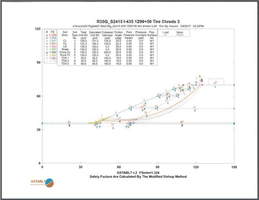
Figure 4 - TDA Slope Analysis Without Lower Soil Layer
