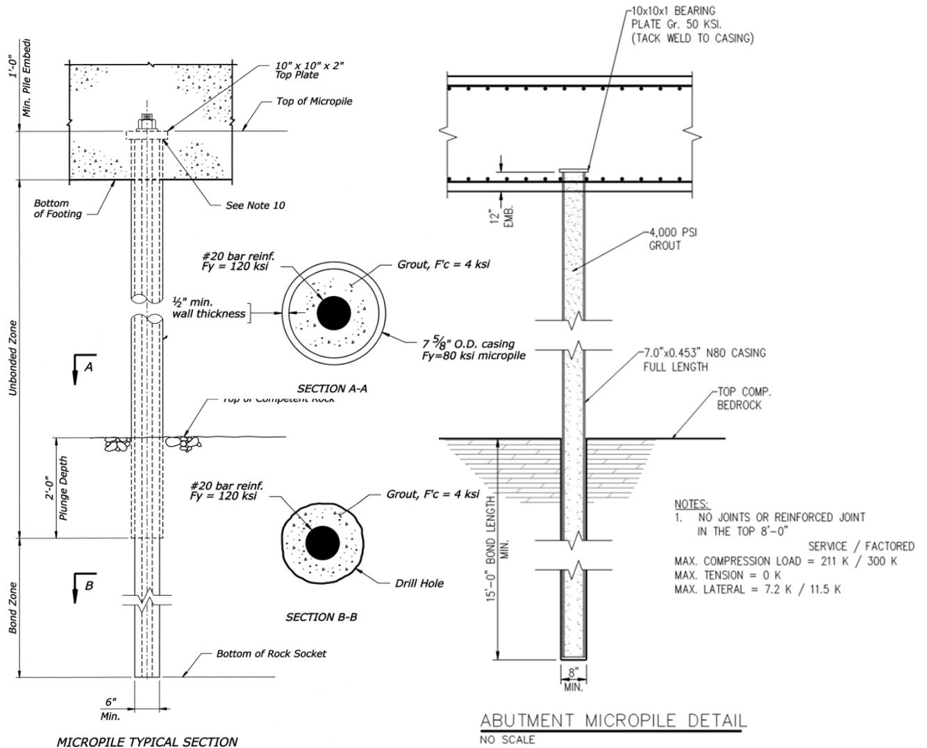
Figure 5 – Design vs. Value-Engineered Micropile Details
