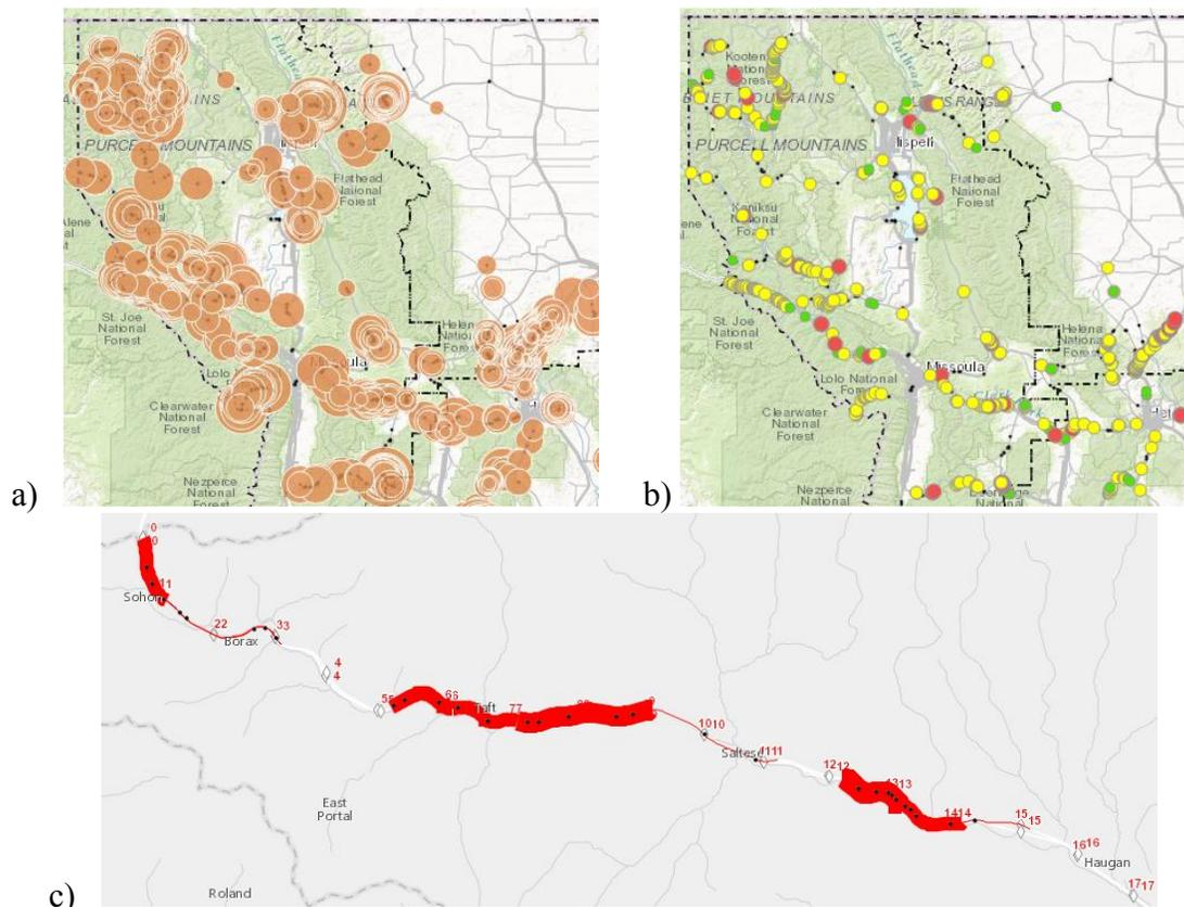
**Figure 7: Screens of NW Montana of a Conceptual RAMP Cloud-Based GIS Interface. A) Total RHRS Score, B) Good/Fair/Poor Classifications, and C) Risk at I-90 near Idaho.**
