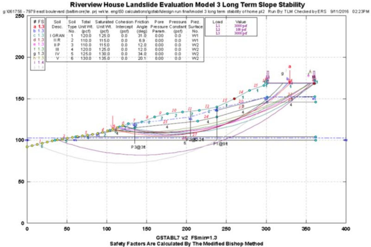
**Figure 7: GSTABL Analysis Landslide Stabilized with ASI Wall 1 and 2**
