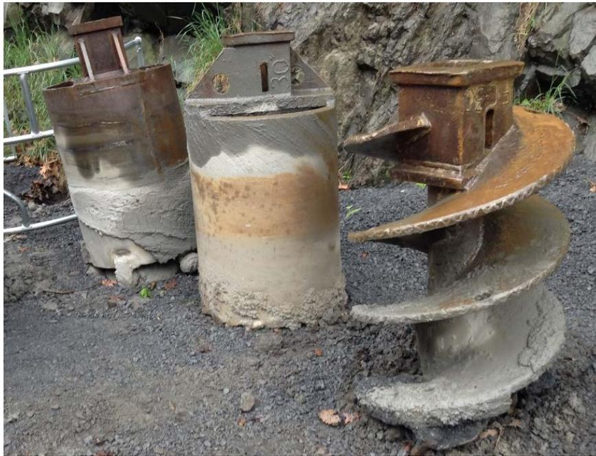
**Figure 7 – Caisson Drilling Tools**
