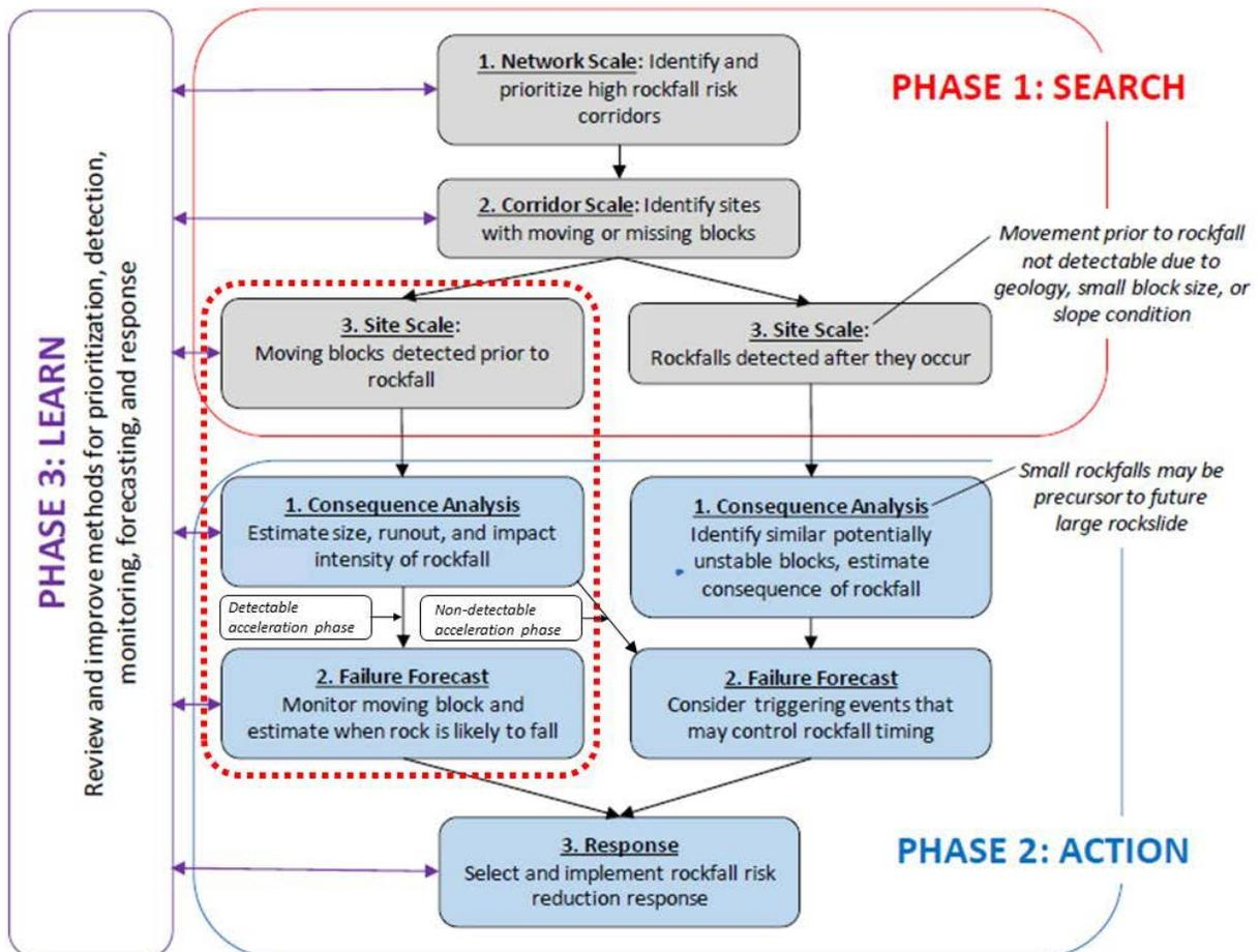
Figure 1 – Framework for rockfall forecasting (adapted from Gauthier et al. 2016)
