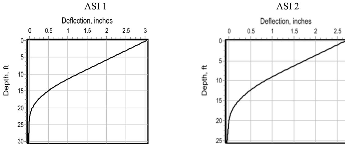
**Figure 8: LPILE calculated Deflection of ASI 1 and 2**
