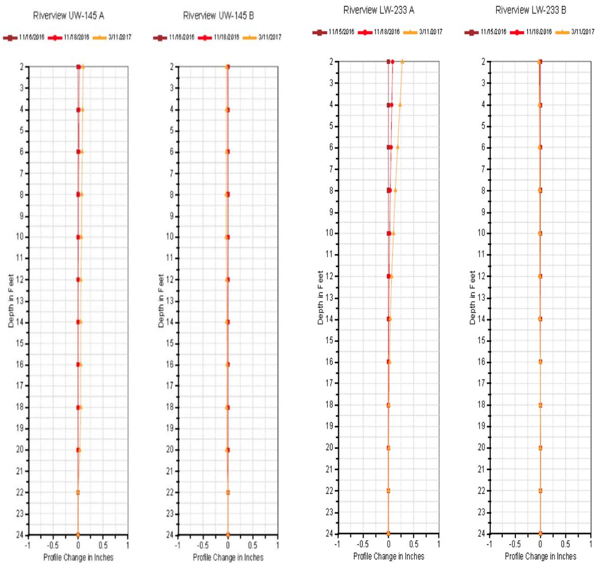
**Figure 5: Post Construction Inclinometers**
