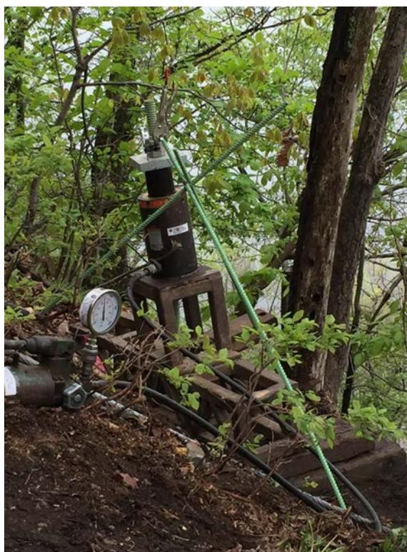
10. Anchor verification test setup
