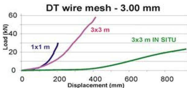
**Figure 6** – Load-displacement curve for tests carried on with different configurations of constraints.
