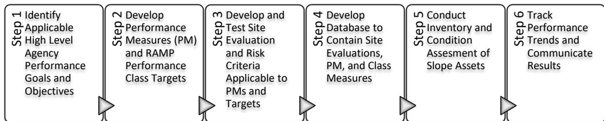
**Figure 3: Flow Chart for RAMP Process.**
