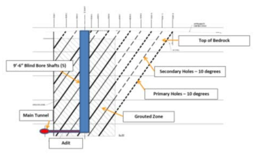
Figure 10. Cross-section view of the pre-excitation grout holes.
