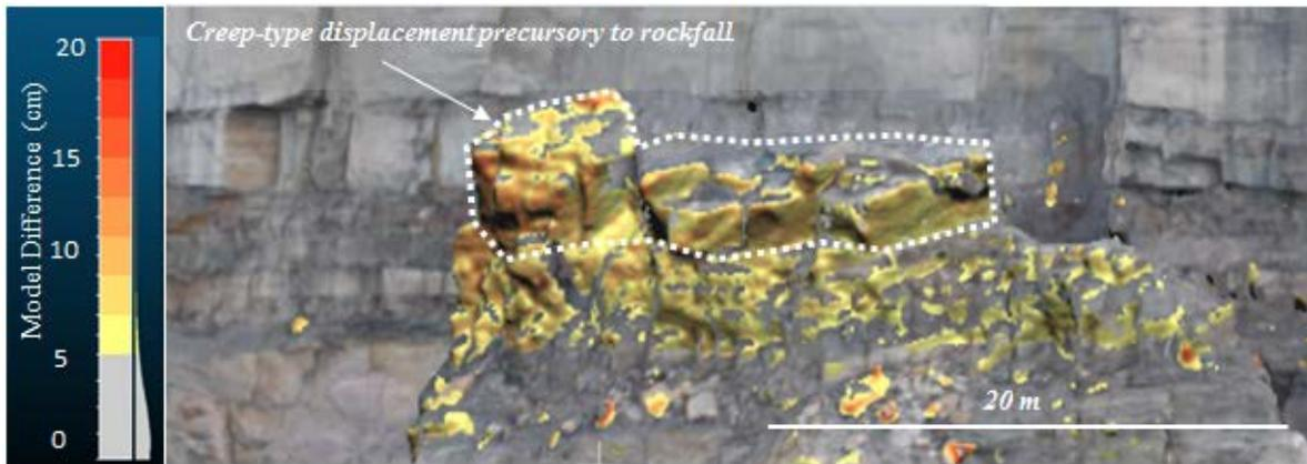
**Figure 4 – Inset from Figure 3. OAP change detection map showing model difference between 5 and 15 cm (adapted from Christiansen et al. 2016)**
