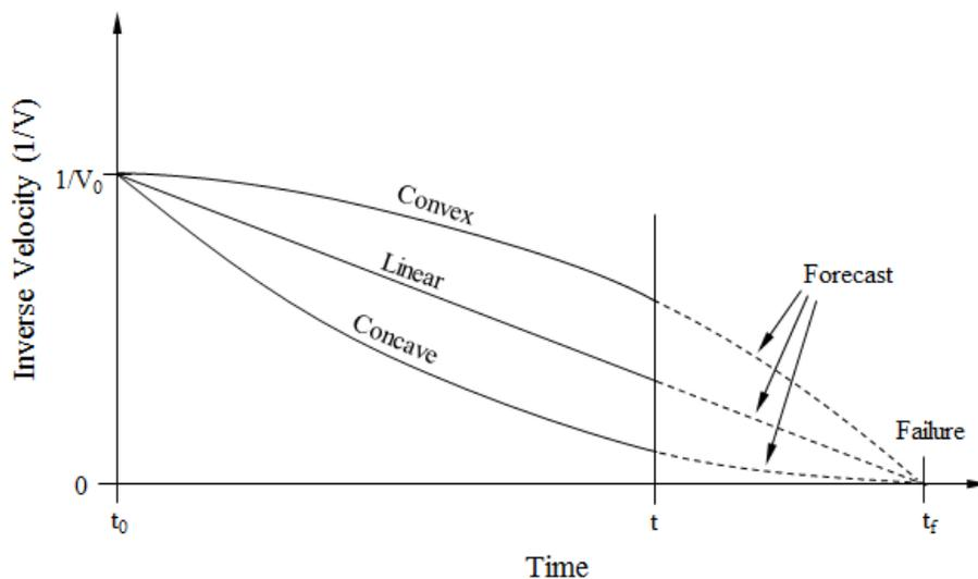
**Figure 5 – Schematic for inverse velocity versus time plot leading up to failure (adapted from Fukuzono 1985).**
