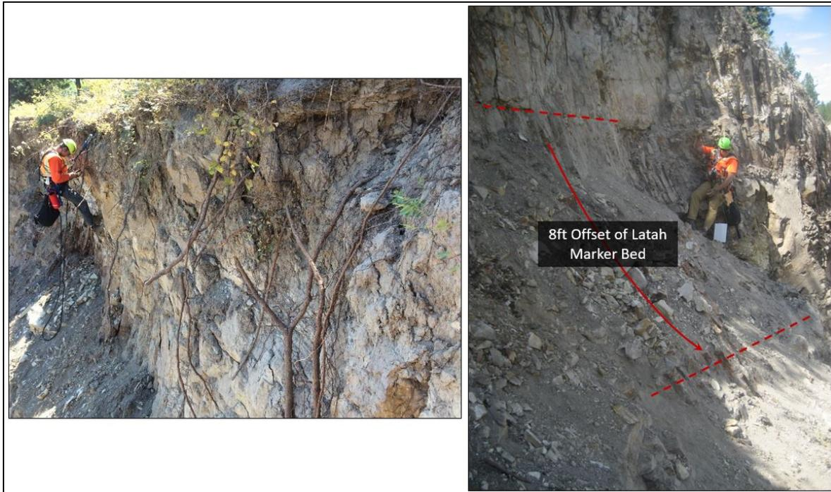
**Figure 6 – Exposed root system penetrating the brow of the slope (left). Interpreted offset of Latah Formation along arching failure plane (right).**
