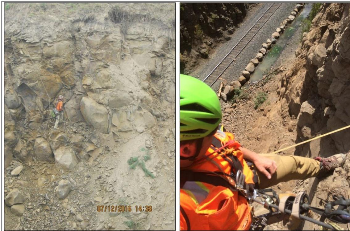
**Figure 4 – Spheroidal weathering of Priest Rapids basalt; note the size of basalt boulders (left). Mapping scanline #3 with rope access techniques (right).**
