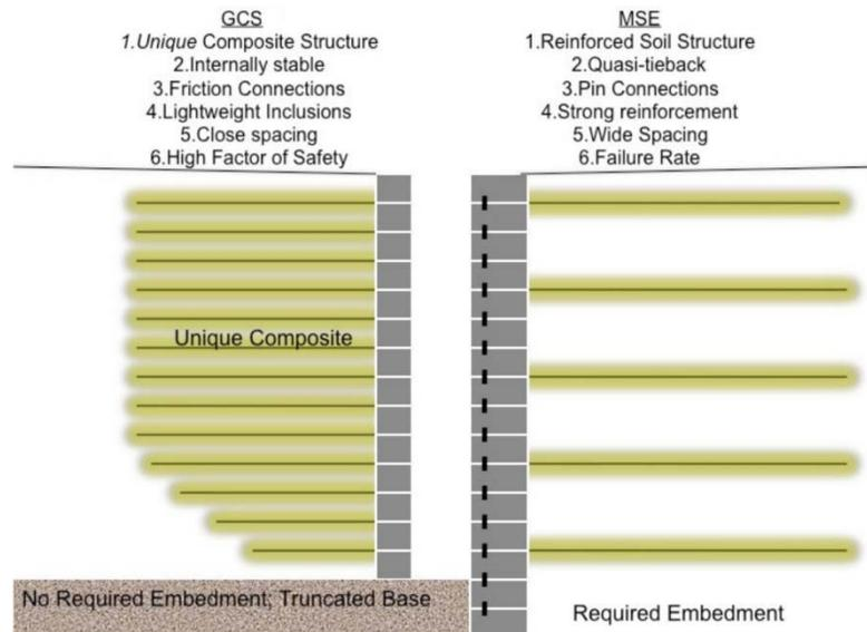
**Figure 1: Differences between GCS walls and MSE walls (3)**
