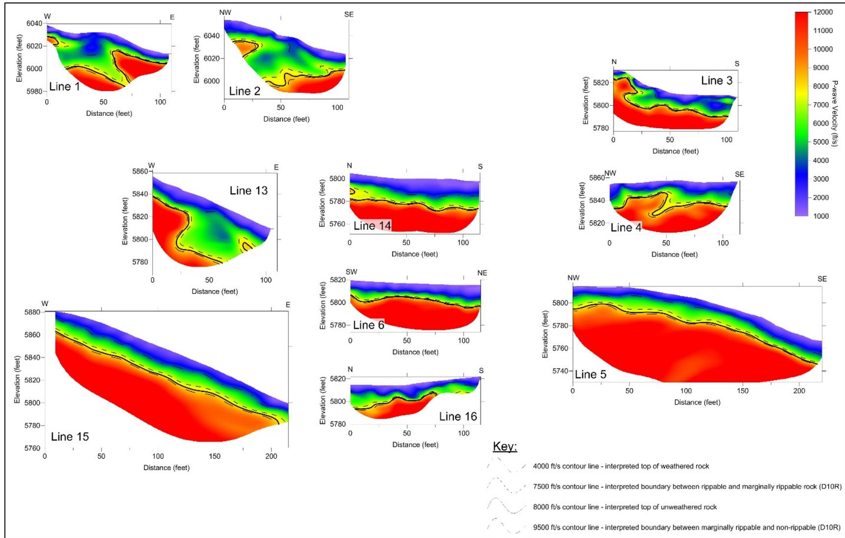
Figure 12. SRT Results from first seismic survey; in the west and central area of investigation.
