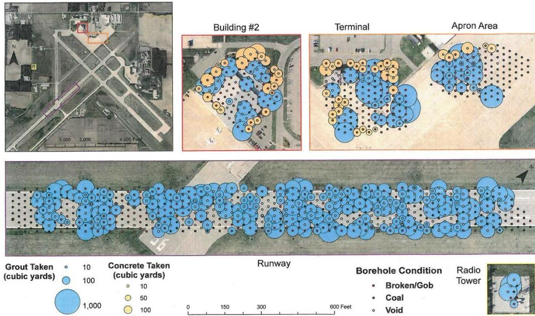
**Figure 4. Borehole 3 Condition, Grout and Concrete Distribution at Terre Haute Airport**
