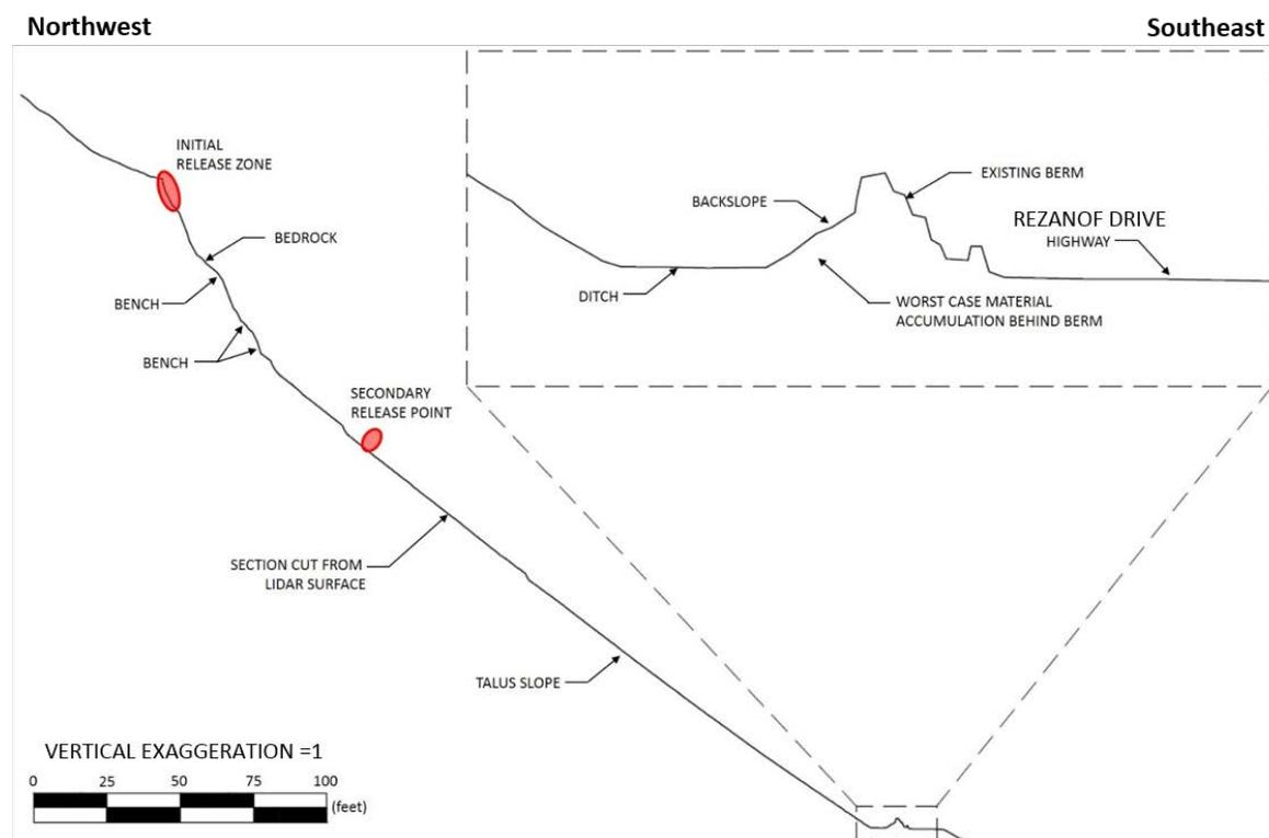
**Figure 6 – Rockfall Modeling Section and Analysis Setup for Calibration**
