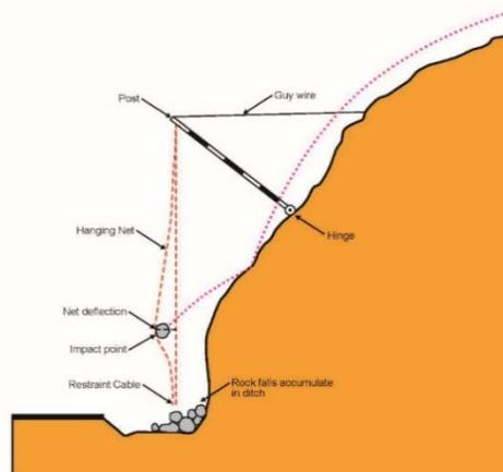
**Figure 1. Typical Attenuator configuration**
