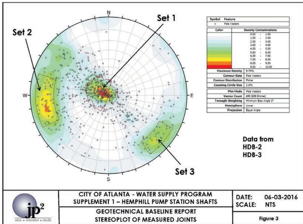
Figure 7. Stereoplot from the Geotechnical Baseline Report of geophysical information showing the high angle joint sets.
