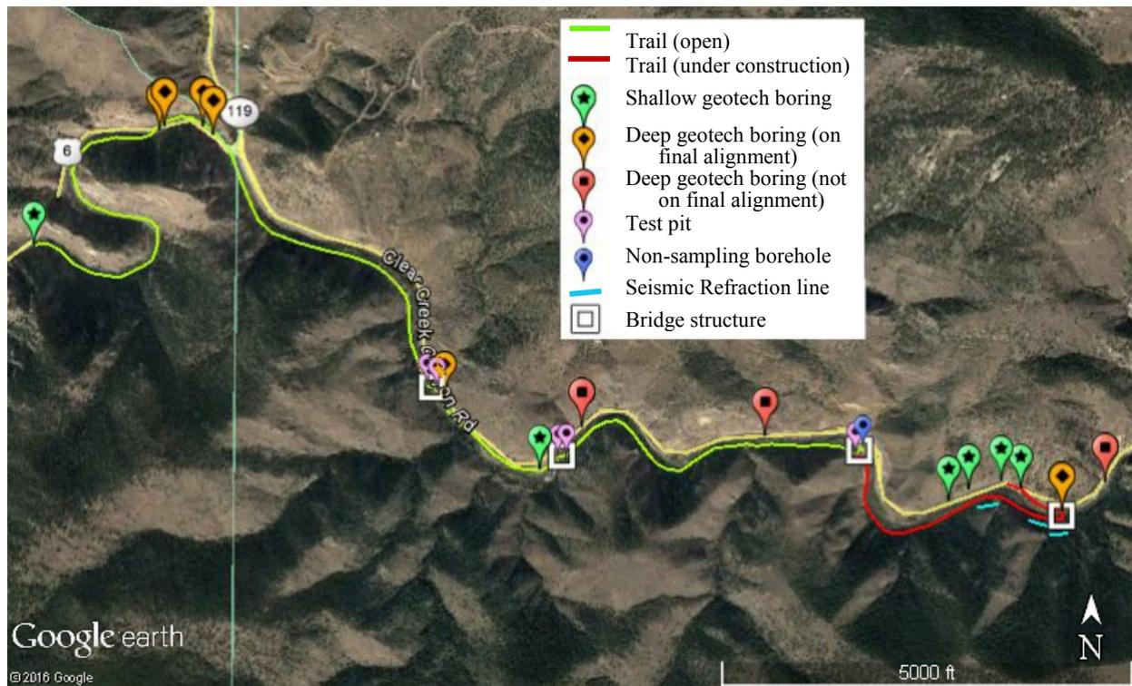
**Figure 7 – Locations of all subsurface geotechnical work. (Not all non-sampling borings are shown for clarity)**
