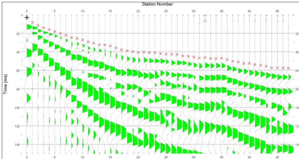
**Figure 7. Example of first arrival picking, indicated by red crosses, from a seismic line collected during the first investigation in the Big Thompson Canyon.**
