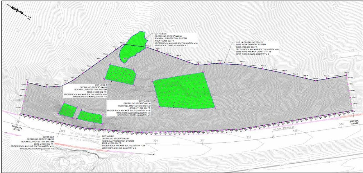
7. Final plan for Southern highwall using tensioned Spider mesh overlaid with TECCO drapery
