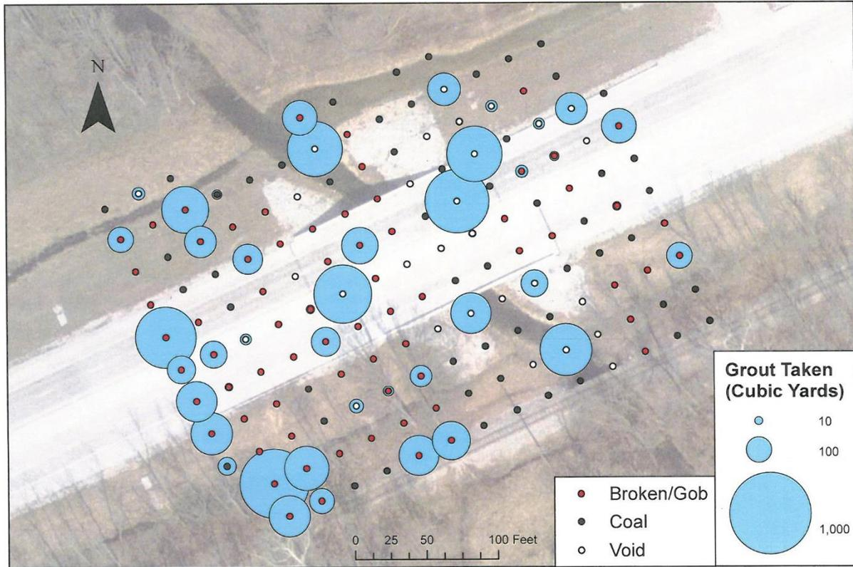
**Figure 5. Borehole Condition and Grout Distribution at the State Road 62 Bridge in Warrick County, IN**
