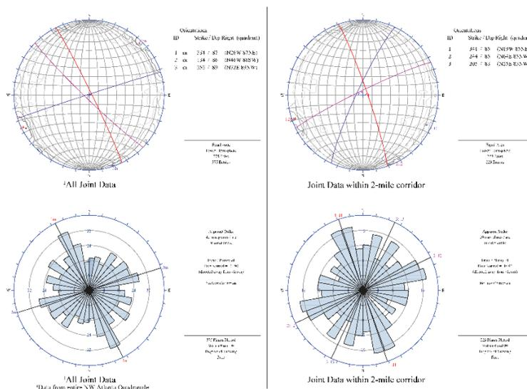
Figure 8. Equal-area stereonets and rose diagrams of measured joints.
