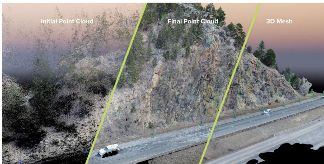
Figure 1. Point-Cloud Processing Workflow Used to Develop a Three-Dimensional Mesh (2)
