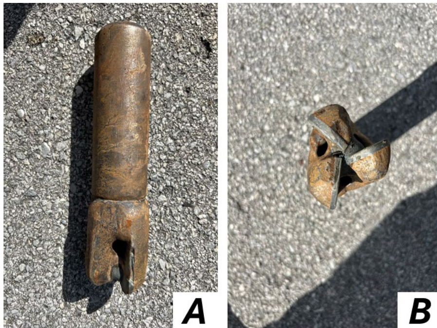
Fig. 6 – Drag bit used by NCDOT for MWD borings showing minimal wear
