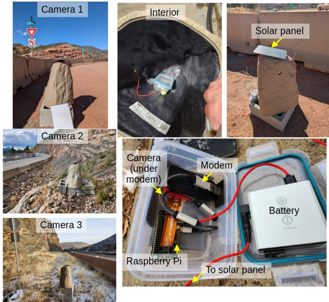
Figure 1 – (Left) Overview photos of the camera installation locations. (Right) Inside view of the camera system enclosure, showing the main components.
