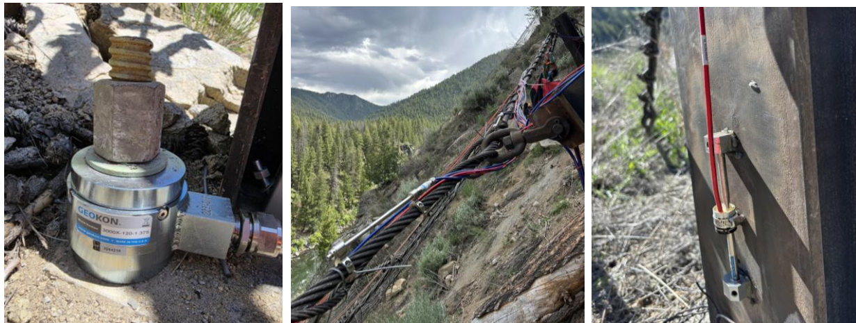
Figure 10 – Anchor Load Cell (left), Top Rope Strandmeter (middle), VW Strain Gauge (right)
