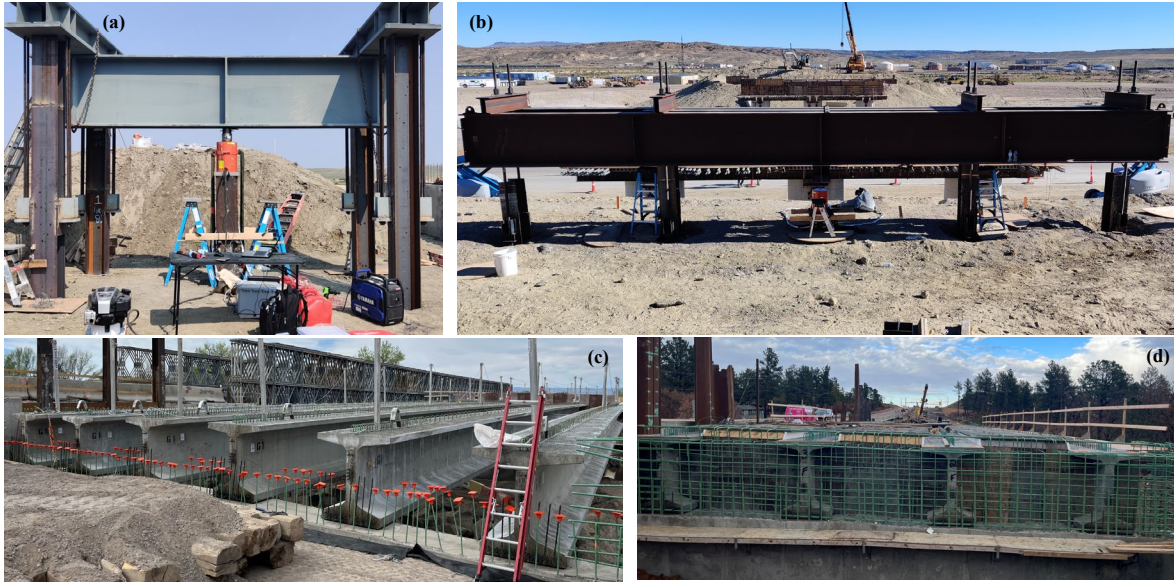
Figure 2. Photos of three static load test systems: (a) IndeSPLS for TP1 to TP5, (b) InteSPLS for TP6 and TP7, and (c) InnoSPLS for TP8 to TP11.
