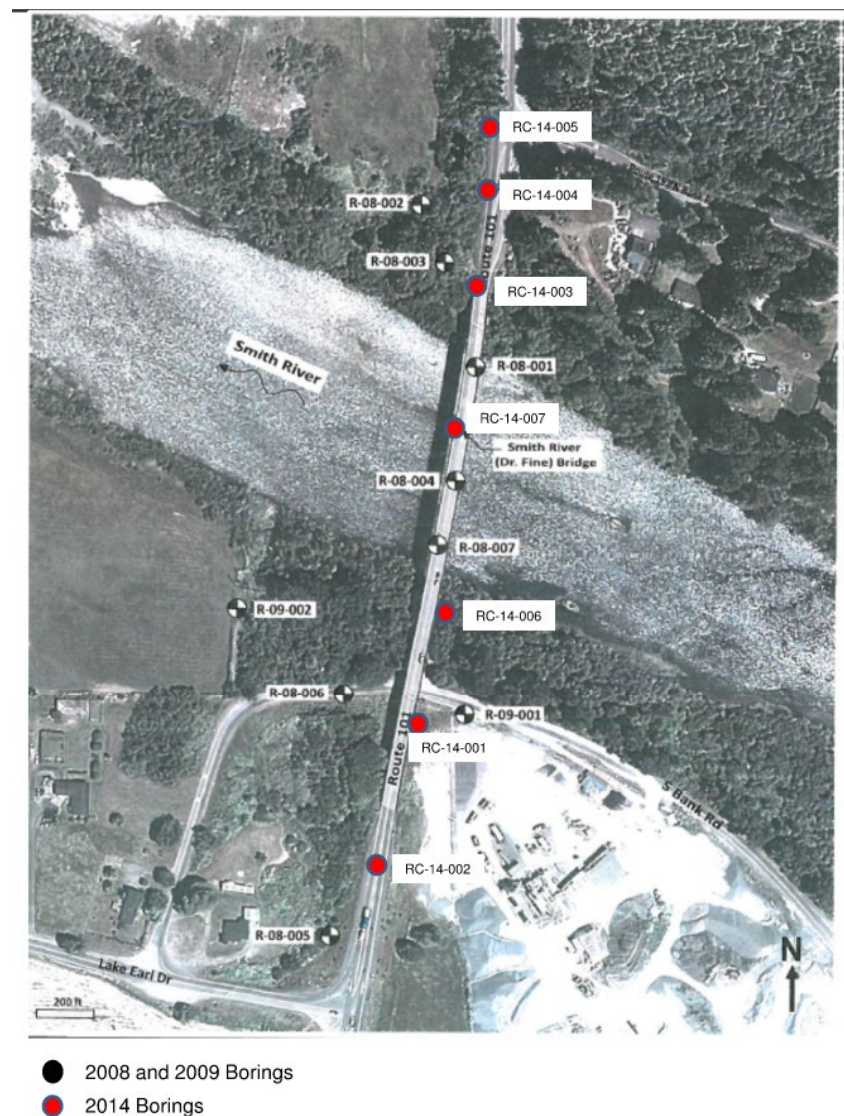
Figure 1: Project and boring location map
