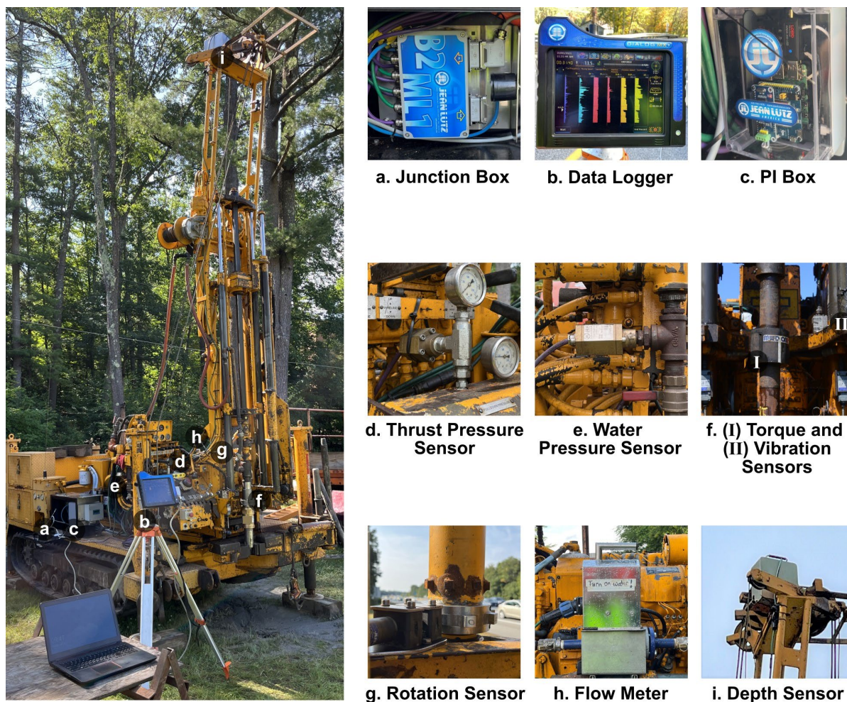
Figure 1. MWD equipment installed on a track-mounted CME-45C drill rig.
