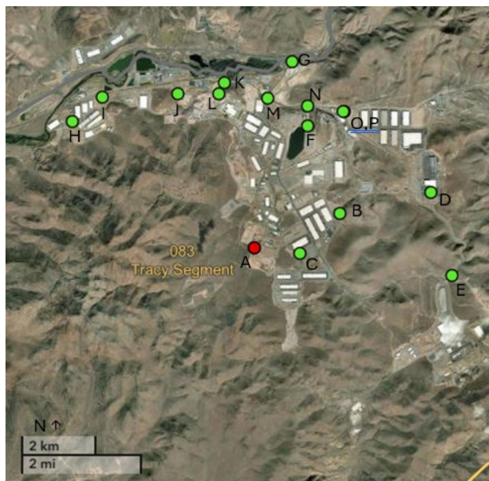
Figure 2. Groundwater monitoring locations within the Tracy Segment Groundwater Basin (Basin 083) near the Tahoe Reno Industrial Center. Green symbols indicate active monitoring sites and the red symbol indicates an inactive monitoring site. Map obtained from the Nevada Division of Water Resources Water Levels Dashboard, accessed July 2026. Well labels correspond to hydrographs presented in Figure 3 and Appendix A.
