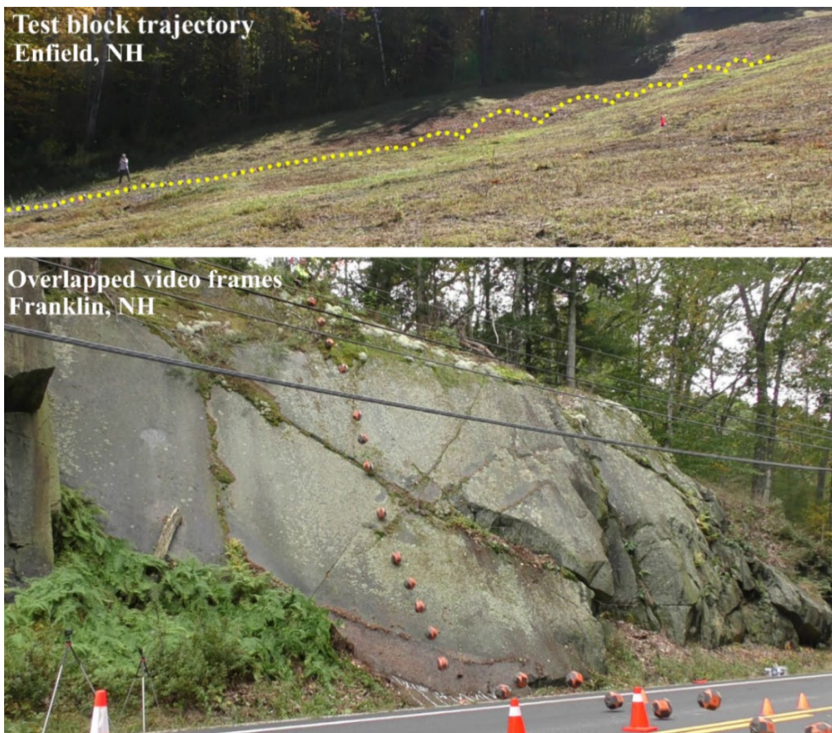
Figure 10 – Field tests in Enfield and Franklin, NH.
