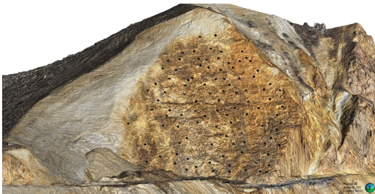
Figure 12 - Perspective View in Leapfrog Works (5) Looking North at Installed Rock Bolt Locations (Black Dots) as Surveyed in the West Cut (imagery and topography collected October 6, 2024, and provided by Granite Construction Inc.).
