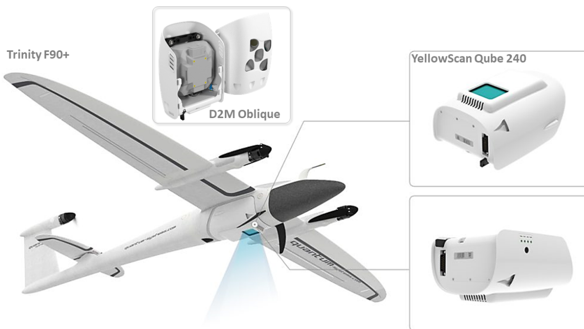
Figure 4 –Trinity F90+ platform, Yellowscan Qube 240 LiDAR sensor, and D2M Oblique camera
