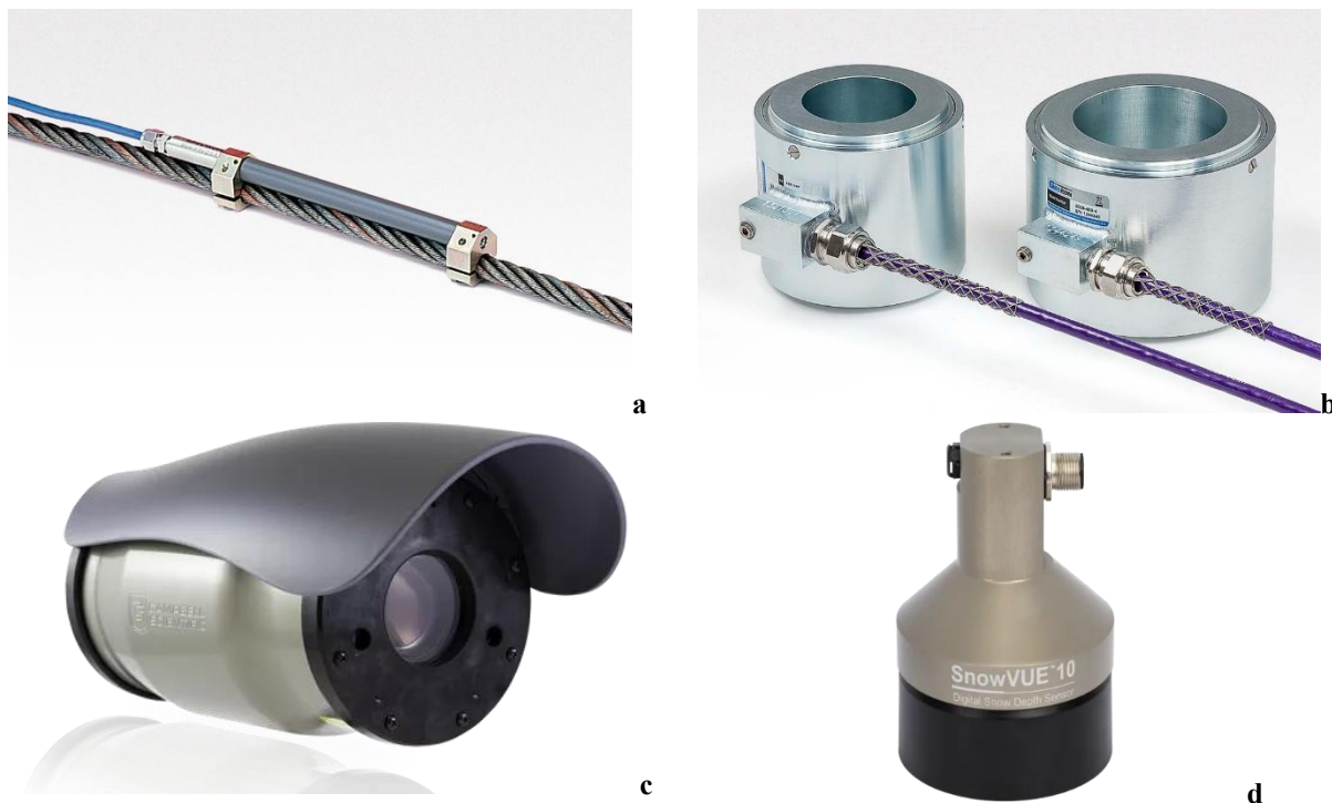
Figure 6 – Images of Strandmeters (a), Load Cells (b), the Camera (c), and Snow Depth Sensor (d).
