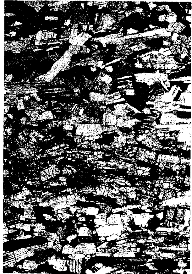
Plate 4. Dolerite/Gabbro. Medium grained interlocking grains of feldspar and pyroxene showing distinct orientation (foliation) with possible banding. (x 8.5)
