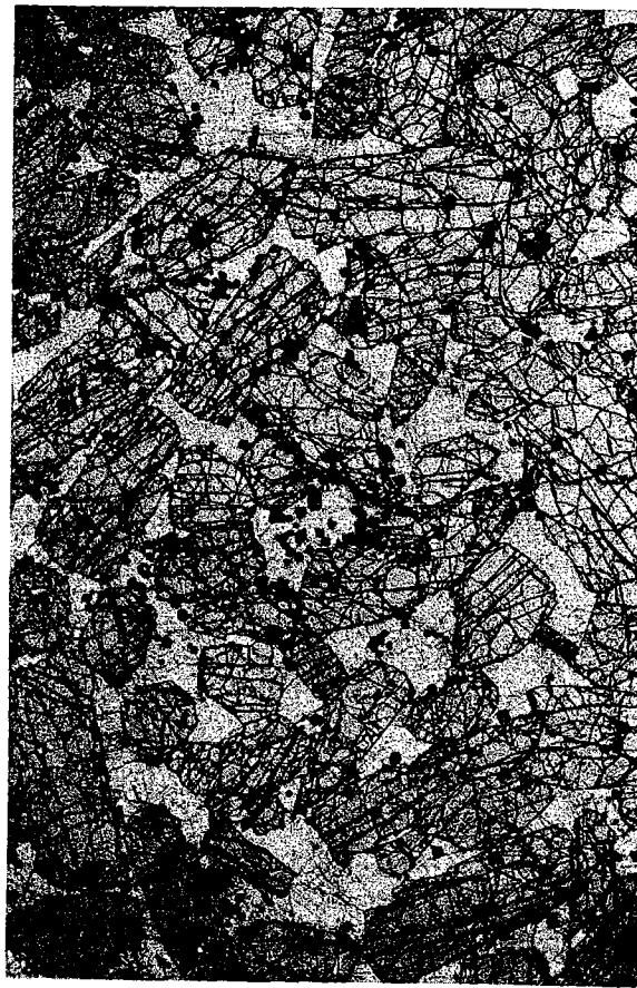
Plate 7. Black specks of finely disseminated metallic ore (Chrome Spinel) occurring in coarse-grained, olivine-rich ultrabasic rock. (PPL x 8.5)
