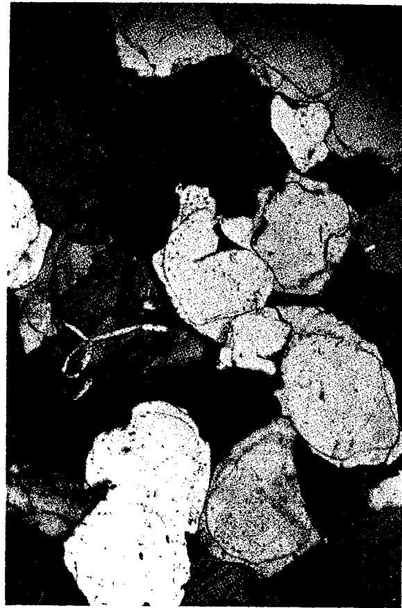
Plate 8. Recrystallized Sandstone (Penrith). Small wind rounded quartz grains cemented together by additional growth of silica from percolating solutions. The quartz jacket is clearly visible. (# x 50)
