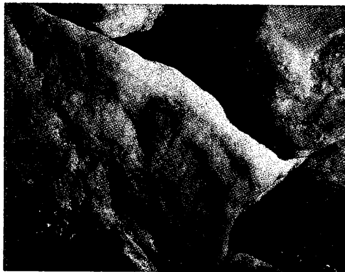
Fig. 8 Close-up of a limestone particle with no microtexture. (Magnification 7X)
