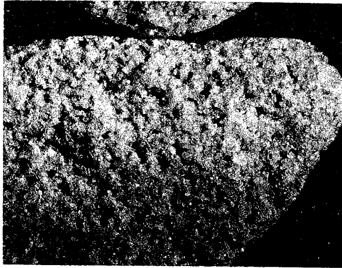
Fig. 9 Sandstone particle showing good microtexture as a result of mineral composition. The sand grains are quartz (Moh's Hardness = 7) and the cementing agent is calcite (H = 3). The polish value measured a 42. (Magnification 7X)
