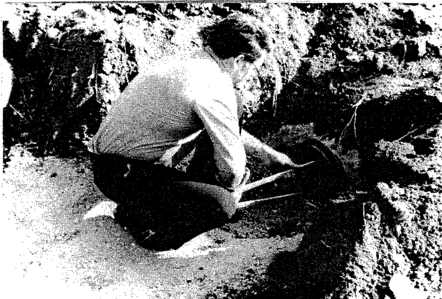
Figure 17. Inside diameters before and after loading were measured by means of a special inside caliper.
