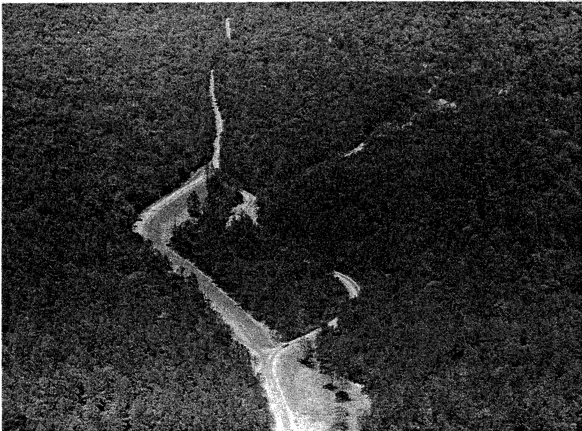
Figure 18. Relocation was the means used to correct the problem shown in Figure 13. The new alignment is at the left.
