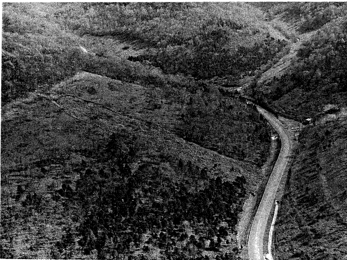
Figure 19. Relocation and re-routing of surface drainage were the methods used in the correction of this slide in Putnam County (see Figures 14 and 15).
