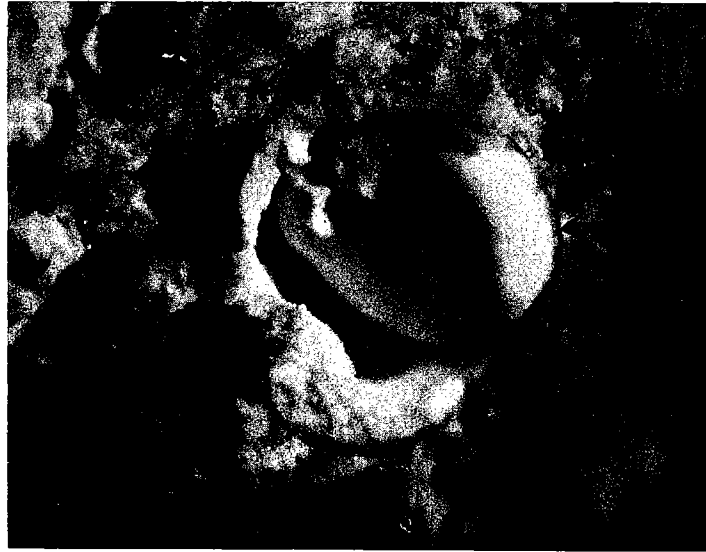
Figure 4. Alkali-silica deposit formed as the result of certain siliceous aggregates chemically reacting with the alkalis in portland cement concrete. Expansive forces capable of disrupting and cracking concrete may result from these reactions. (Magnification 25X)
