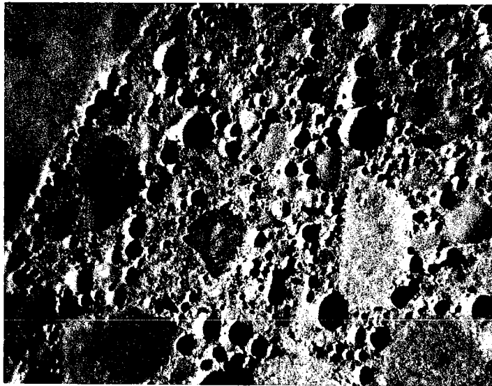
Figure 11. An entrained air system measuring 14.5 percent by volume. The spacing factor is 0.002 inches. (Magnification 20X)
