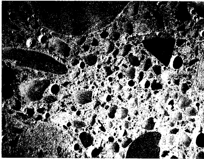
Figure 10. An entrained air system measuring 3.2 percent by volume. The spacing factor is 0.75 inches. (Magnification 20X)
